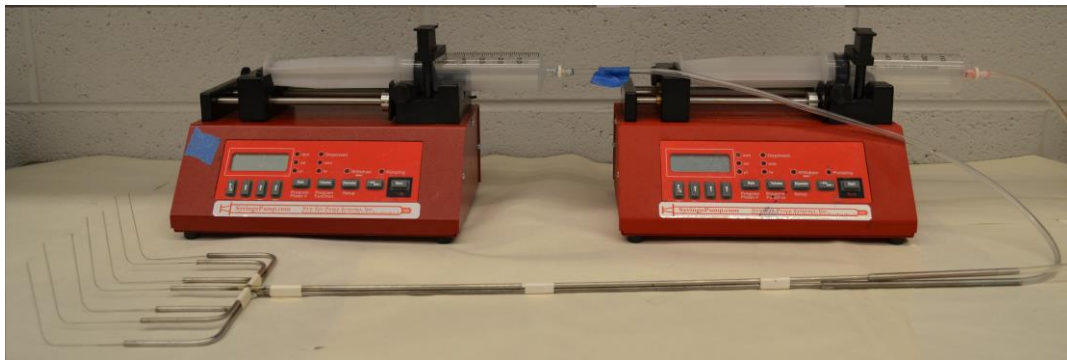
Figure 2.14 Instruments for dye injection
