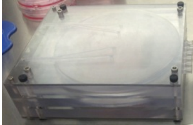
Figure 5.4 Flip Plate Bioreactor System. Approximate dimensions are 7 in x 6 in x 2 inches.
