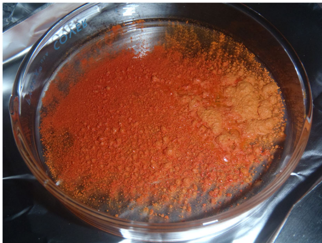
Figure C.9: Heating of dried uranyl nitrate to 300 °C for two hours is believed to have resulted in conversion to \text{UO}_3 , as evidenced by the orange coloration.
