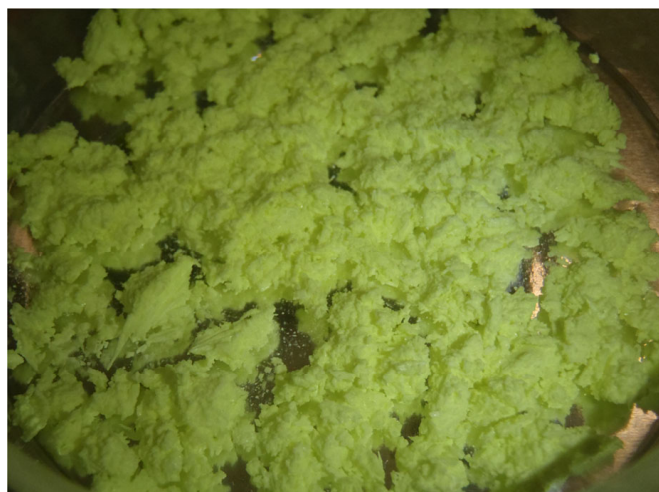
Figure C.8: Dehydration of uranyl nitrate crystals above lithium chloride in a desiccator led to a substance with constant mass, but an uncertain hydration state.
