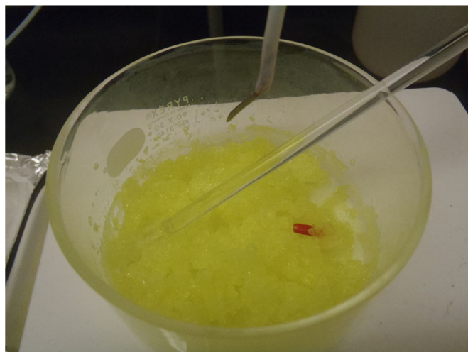
Figure C.7: Dehydration of uranyl nitrate resulted in the formation of yellow crystals presumed to be uranyl nitrate hexahydrate.
