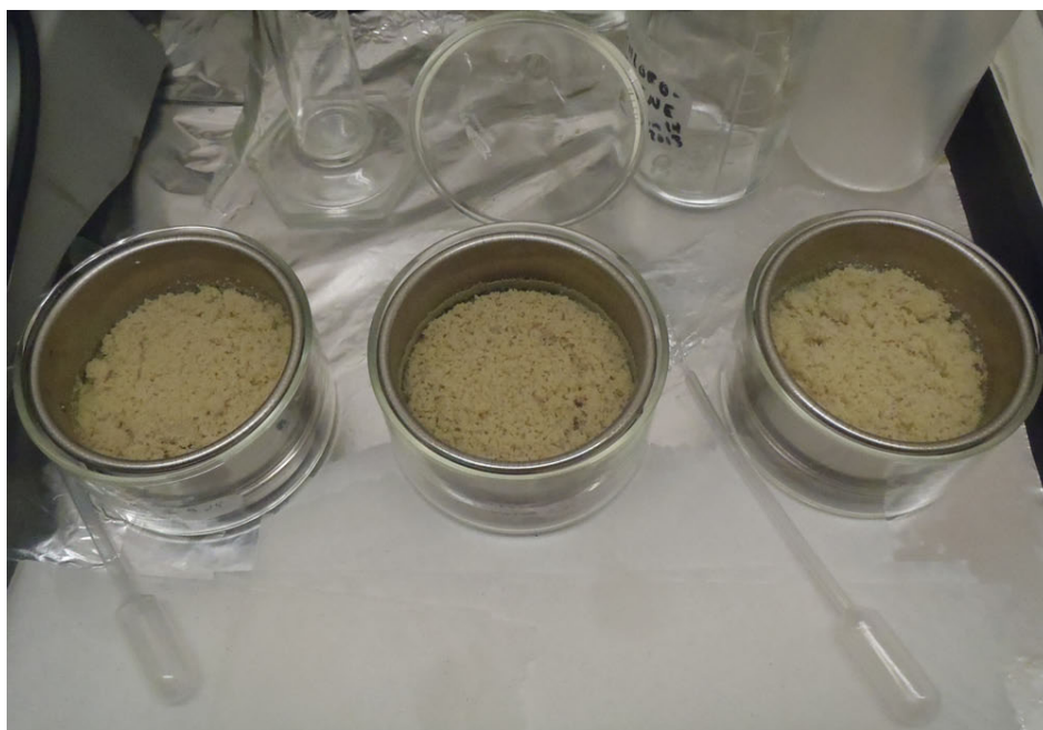
Figure 4.11: Three batches of microspheres were washed in separate mesh sieves held in glass dishes.
