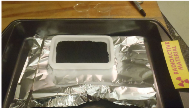
Figure C.1: Uranium oxide powder was heated at 600 °C for two hours for conversion to U_3O_8 .
