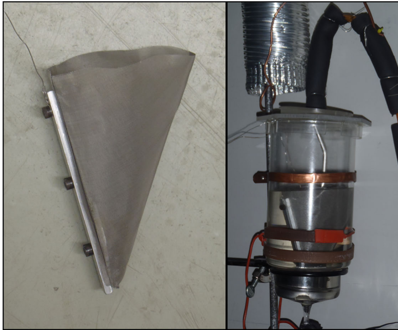
Figure 3.14: After exiting the column, microspheres pass through serpentine tubing and collect in a conical mesh basket.
