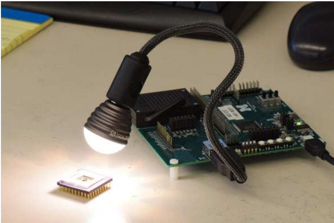
Figure 5.19: Proposed system being programmed via light.
