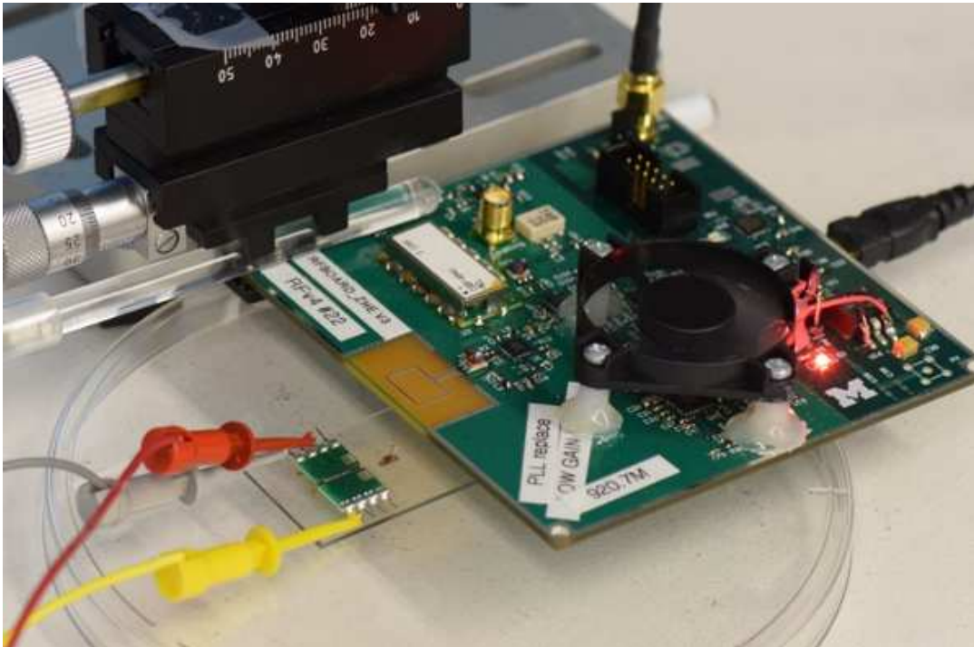
Figure 5.20: RF reception testing setup.
