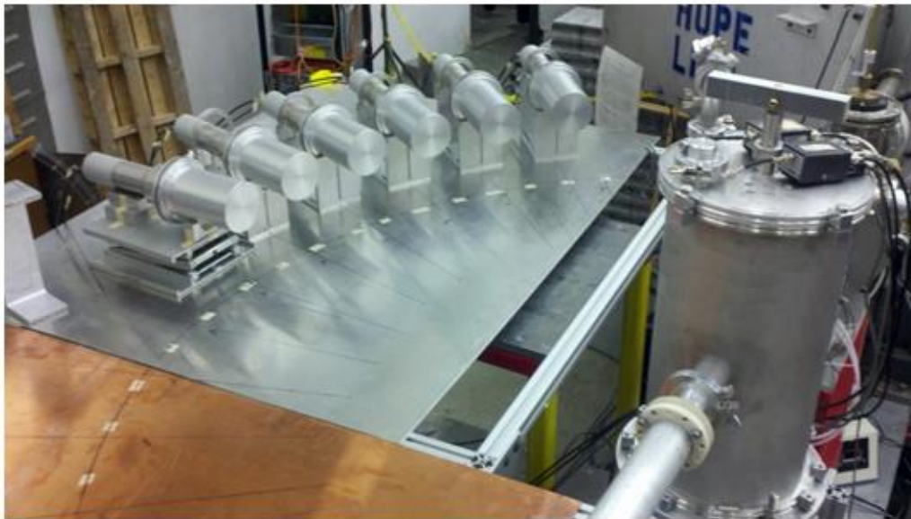
Figure 6.2 - The experimental setup used in the (d,n) measurement campaign. The 4x6 EJ-315 detectors shown are positioned 1 m from the target.
