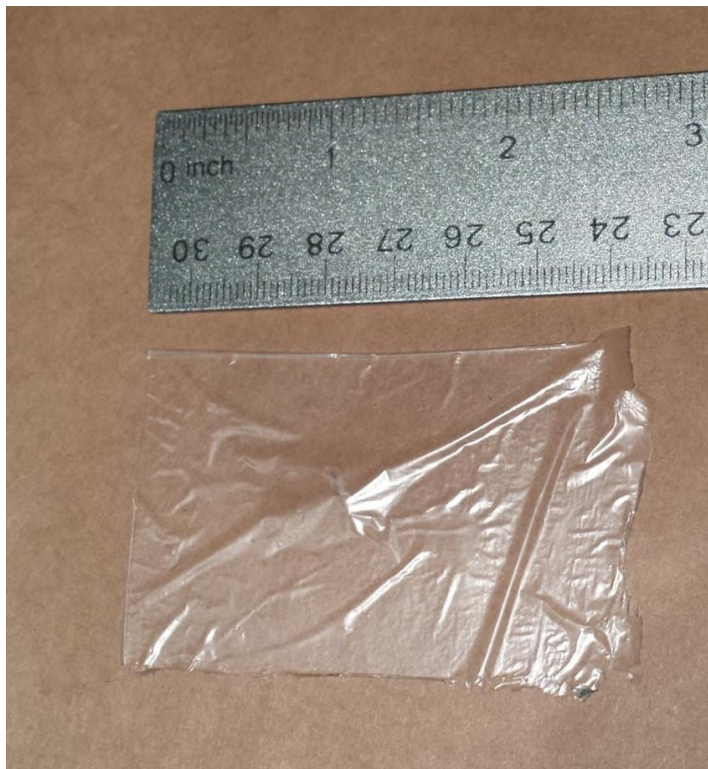
Figure F.2 – A finished large-area deuterated polyethylene target
