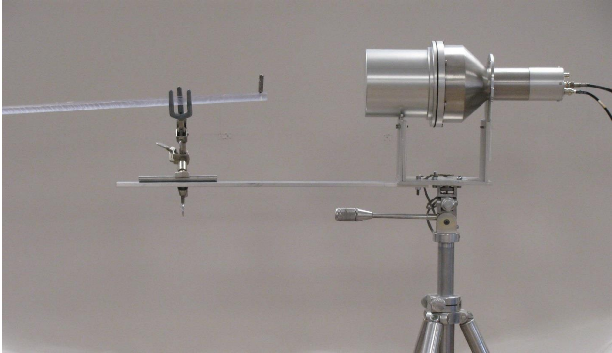
Figure 6.8 - Experimental setup for the PuBe measurement showing the 5x5 EJ315M scintillator mounted on a tripod stand. 1.27 cm lead plate not shown in figure.
