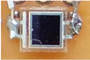
Figure 4.20 Wide-range light sensor installed on the south wall of the test building
