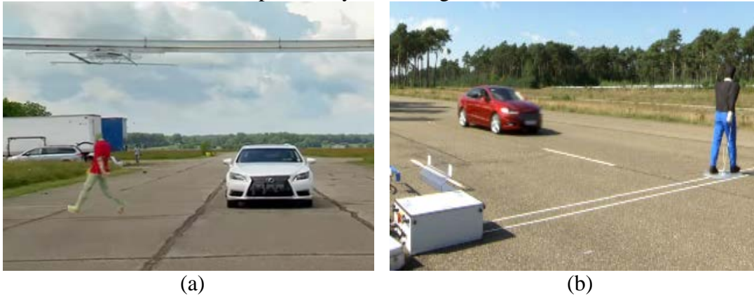
Figure 2: Two different pedestrian testing apparatuses. Toyota uses a mannequin connected to a gantry (a) and Ford pulls a mannequin across a grounded track (b).
