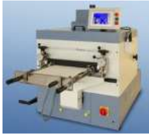
Figure 2: Mathis Labcoater Type <<LTE-S>> coater and drier used in the Battery Lab [11]
