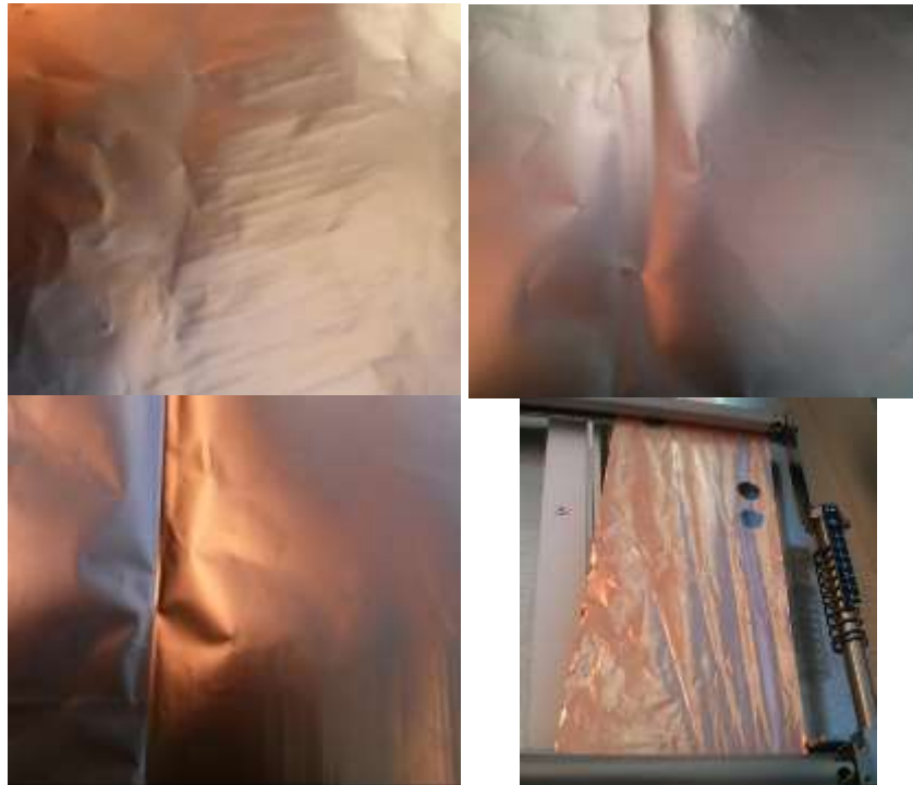
Figure 10: Wrinkle types 1 (top left), 2 (top right), 3 (bottom left), and 4 (bottom right). Wrinkle types 1-3 are caused by handling, while type 4 wrinkles are caused by tensioning. The severity of the wrinkle increases with the value (e.g. type 1 wrinkles are less severe than type 3 wrinkles).
