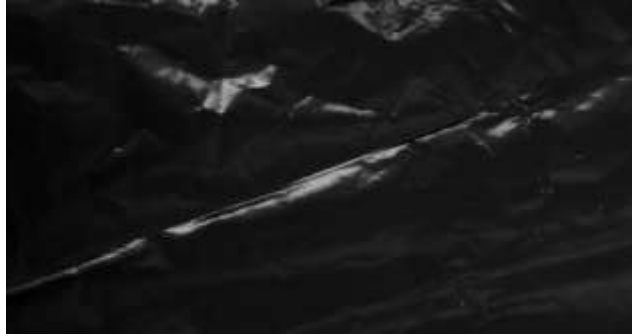
Figure 9: Black and white image of a wrinkle in the foil to be used for 2D image analysis.
