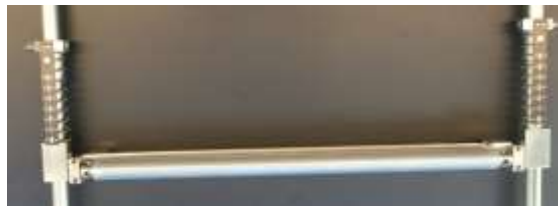
Figure A.4.5: The current tension system fixes the movable clamp on the frame and uses short springs to apply additional tension.
