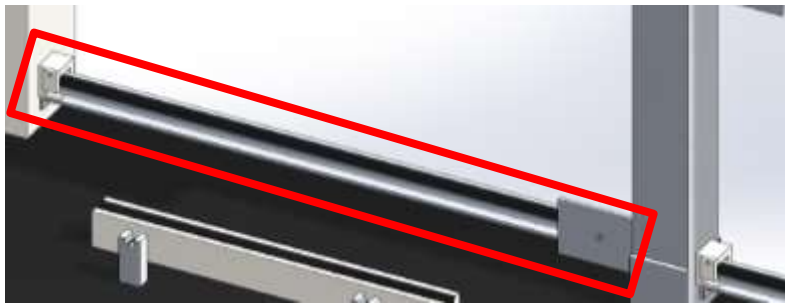
Figure 26: Two non-rolling bars would be placed on top of each other to guide the foil between them and keep it at the correct height.
