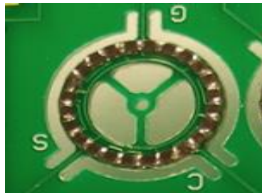
Figure E.1: 13 mm PCB motor stator. It has support inside the stator that can constrain the axis of rotation. Similar design for the stator can be introduced to our design of the stator and eliminate additional shape of cup for the top plate.
