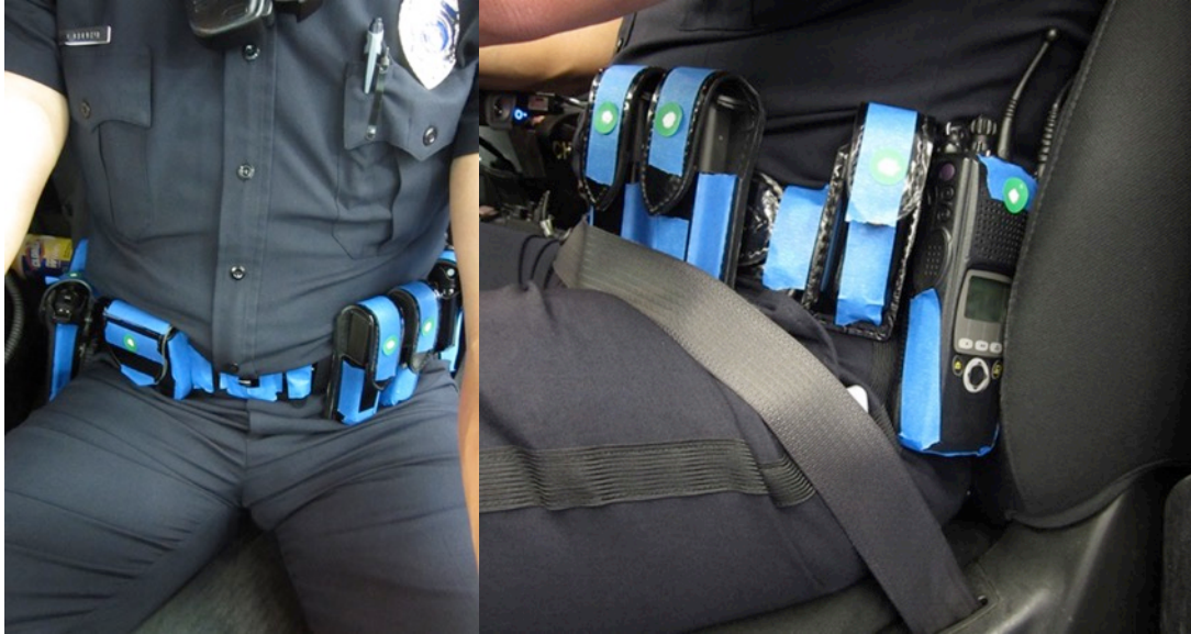
Figure 67. Interference between the duty belt and seatback bolster (L3).
