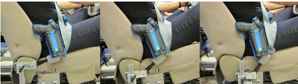
Figure 58. Restraint in mockup with anchorage set relative to H-point at 30°, 52° and 75° which span the range of angles permissible in FMVSS210. Note the routing of the belt.
