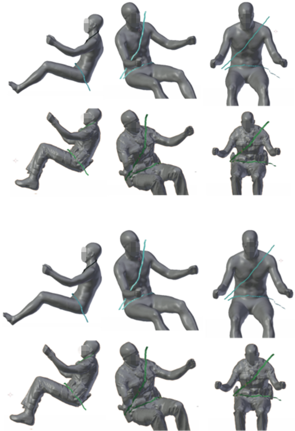
Figure 61. Belt fit visualization using laser scan data and belt routing measured in the vehicle mockup.
