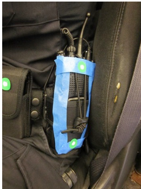
Figure 64. Radio digging into bolster (note seat wear due to equipment contact during ingress).
