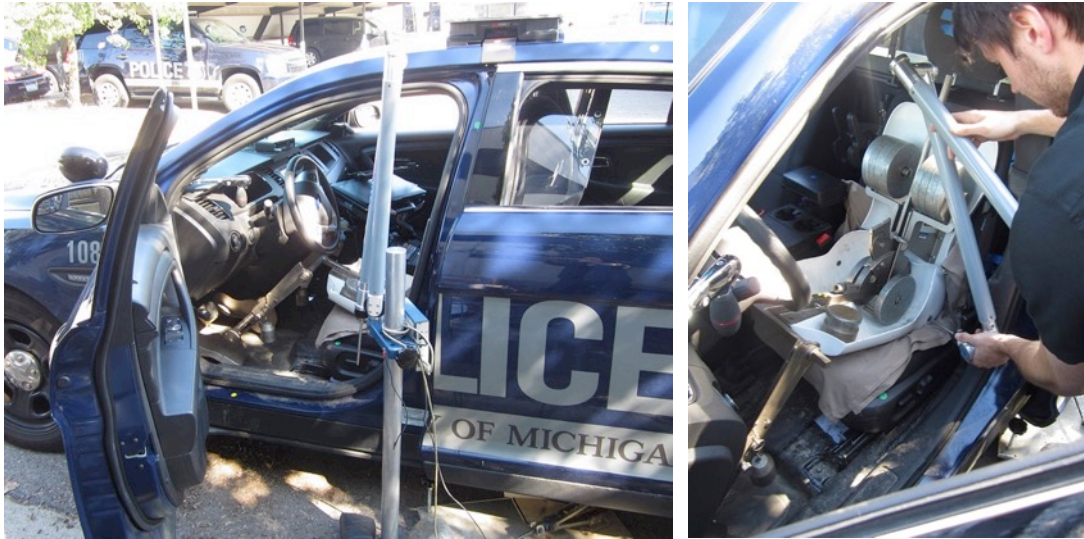
Figure 17. Set up for digitizing the Taurus (left), digitizing the H-point location on the J826 H-point machine in the vehicle (right), as well as detailed measurements of vehicle geometry and package layout.
