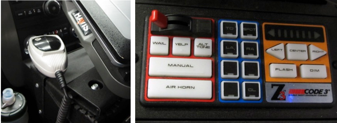
Figure 15. Center console components, which include controls for 2-way radio communication, visual and audible warning systems.
