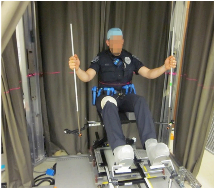
Figure 30. Whole-body laser scanner, with officer in a posture similar to driving. The arms are held away from the body to improve coverage of the torso.
