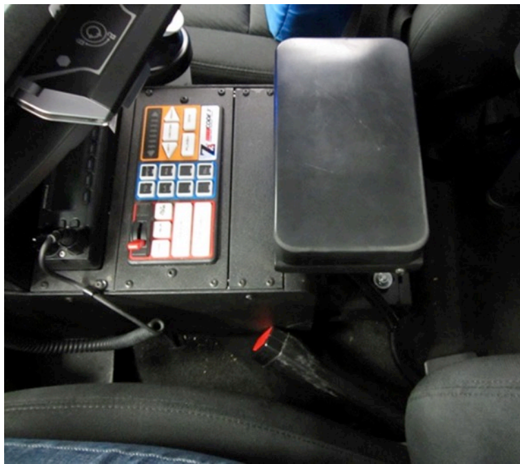
Figure 14. Center console components and mount for mobile data terminal.
