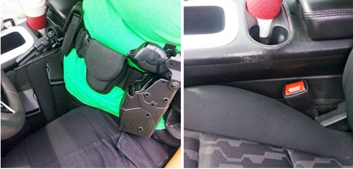
Figure 65. Officer showing interaction between thigh holster and center console (left), which makes donning the seat belt difficult. The belt then covers the weapon making it impossible to draw quickly. The scratch marks on center console from holster (right).
