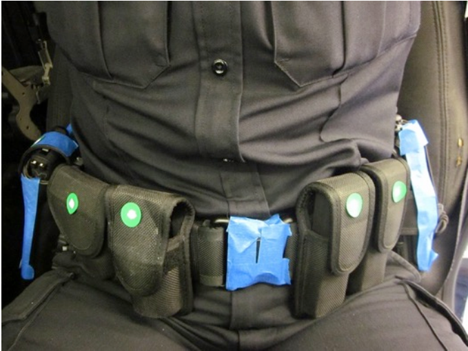
Figure 66. Female officer in Tahoe seat (L2). Officer reports interference of communication radio with seatback bolsters.
