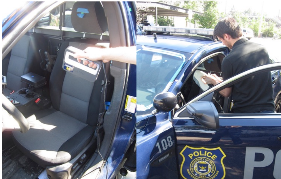
Figure 18. Documenting vehicle interior with hand-held scanners: 3DSystems Sense (left) and Artec Eva (right).
