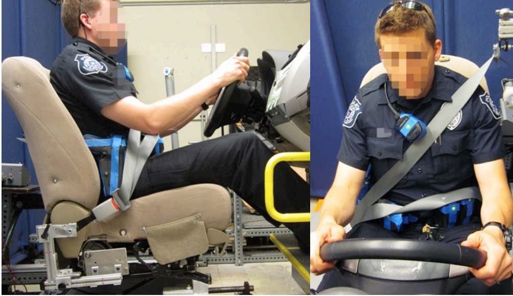
Figure 59. Lower anchorage angle 30° and upper at mid setting. Note the routing of the belt.
