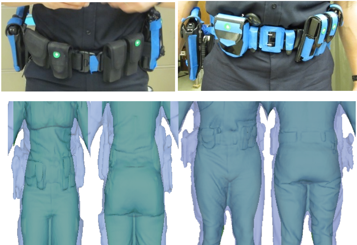
Figure 48. Standing space claim analysis for two officers. The images at the top show the duty belts.
