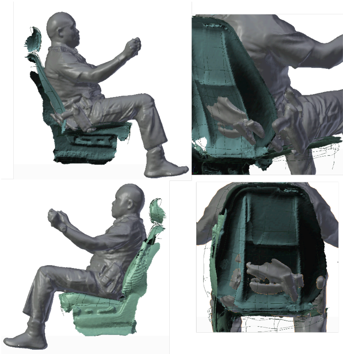
Figure 69. Side arm, flashlight, and mace create pressure point at lower back due to interaction with the seatback cushion and bolster in a Tahoe seat (L1).
