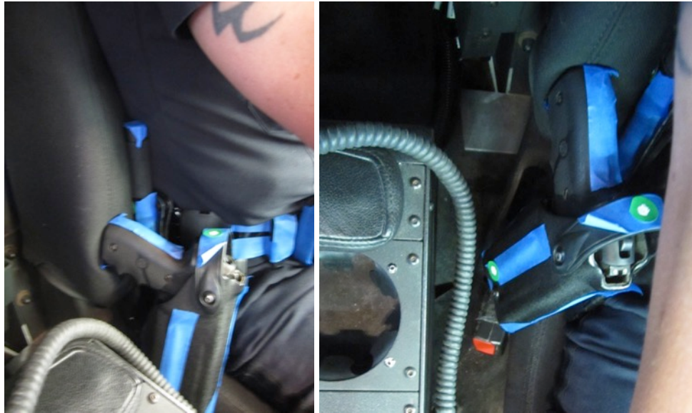
Figure 63. Interference between the duty belt and seatback bolster (left) and center console (right).
