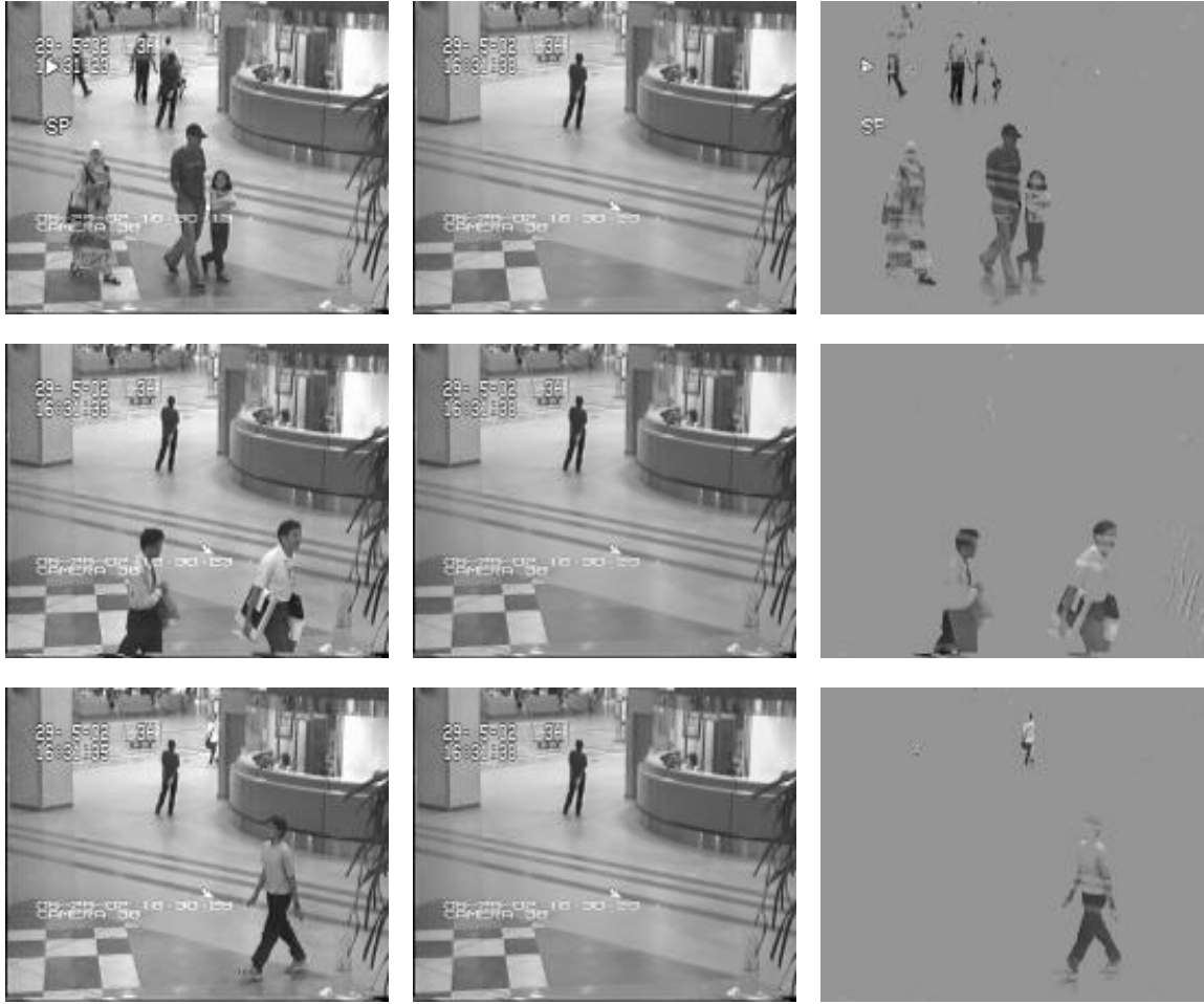
Figure 4.1: The panels describe background modeling from a 200 frame sequence video taken in an airport. The first column shows three original frames. The second and third columns display low-rank \hat{L} and sparse \hat{S} obtained by Algorithm 4.
