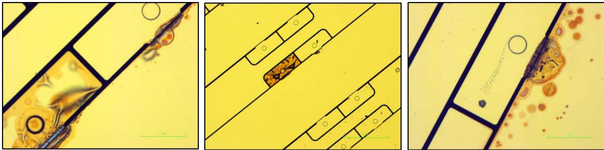
Fig. 8.28. Micro-welding at the electrodes due to excessive current flow.
