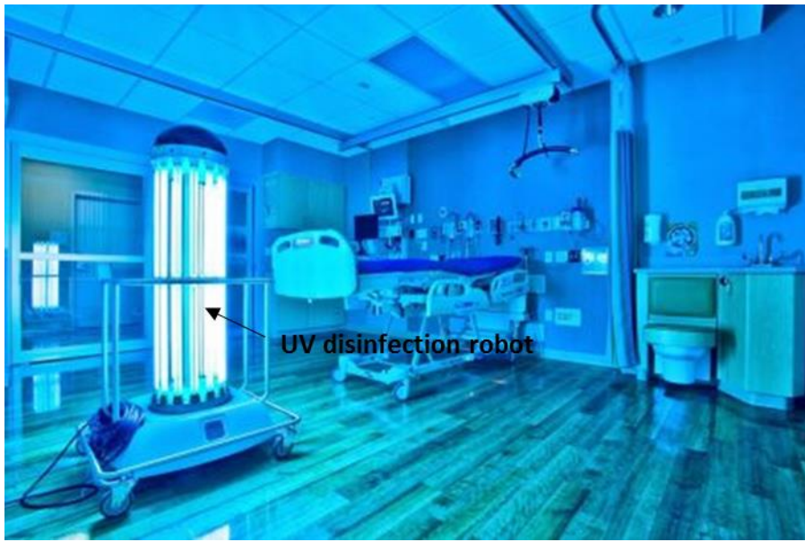
Figure 2.5: A portable UV robotic system that precisely measures reflected UV light and automatically determines the optimal dose required for disinfecting health care environments. [Figure and caption appear in and are taken from [107]]
