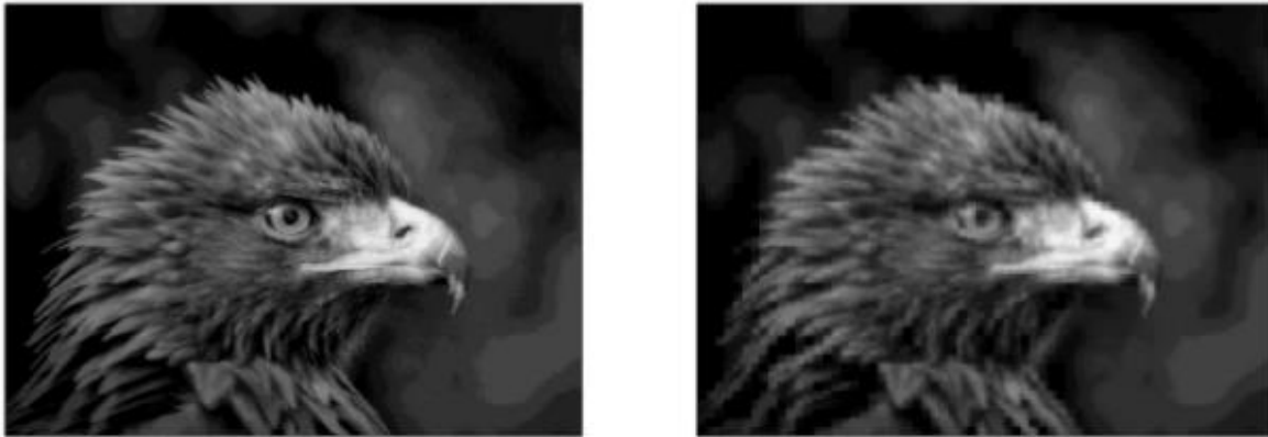
Figure 2.28 640×480 video frame reconstructed using 10×10 patches with a 100×200 memristor crossbar. Left: original. Right: reconstructed.
