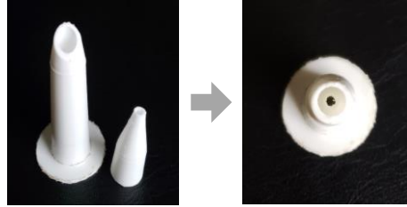
Figure 4.11 Internal nozzle used to achieve a shallower caulk flowrate profile
