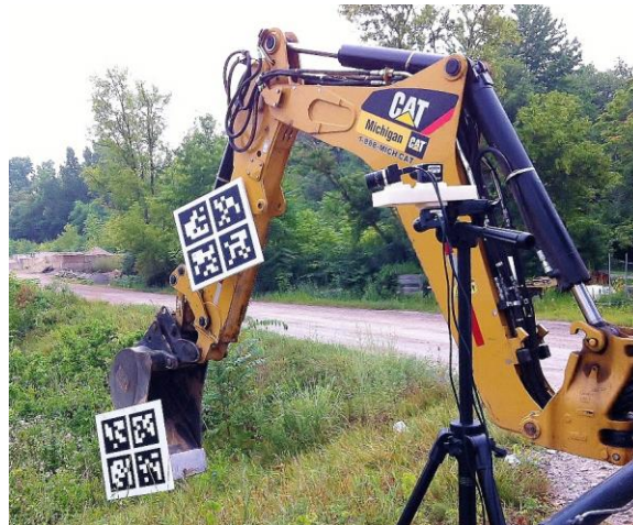
Figure 2.24 Cable potentiometer generalized mapping prototype installed on backhoe
