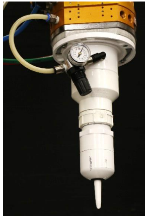
Figure 4.8 Caulk dispensing tool
