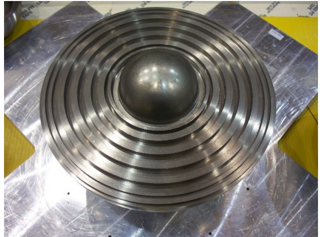
FIGURE 2.1: CAD image of a typical reflected plutonium setup (left), and picture of the BeRP ball within metal reflector shells (right).
