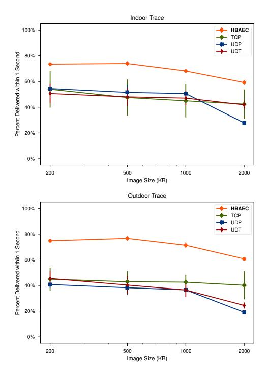
Figure 4.4: Percent of images delivered during trace-driven network emulation for High Bandwidth Adaptive Erasure Coding (HBAEC), Transmission Control Protocol (TCP), User Datagram Protocol (UDP), and UDT. HBAEC delivers a higher percentage of images compared to the other protocols.
