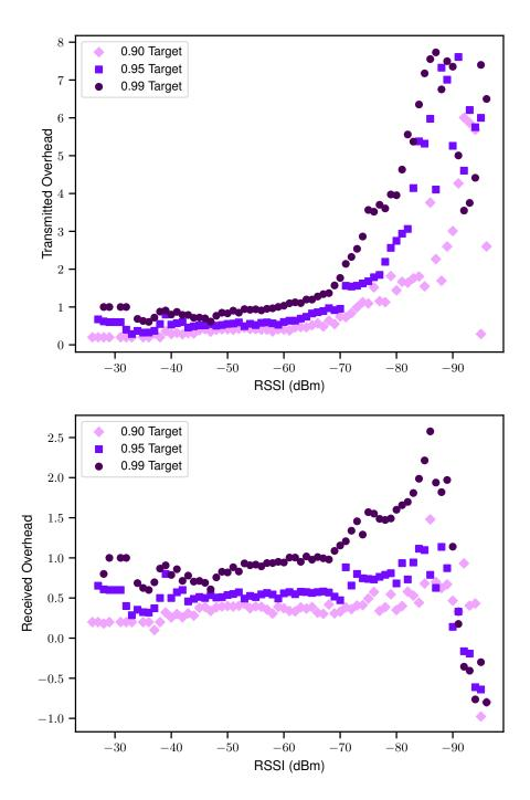
Figure 3.4: Measured overhead needed to achieve packet reception ratio (PRR) results of Figure 3.3. Transmitted overhead (amount of parity transmitted relative to amount of data transmitted) increases as link quality degrades and is greater for higher target PRR levels. Received overhead (number of packets received relative to amount of data transmitted) is also greater for the higher target PRR levels.
