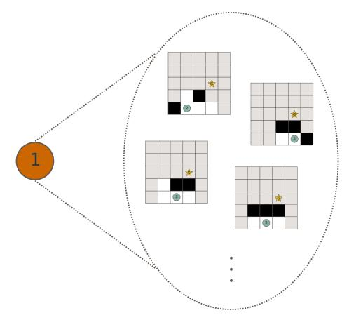
Figure 5.2: An illustration of Robot 1's belief over models of its teammate (Robot 2) in the multi-robot navigation task. These models represent possible locations and maps for Robot 2.
