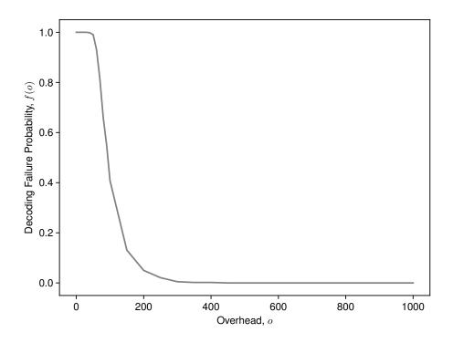
Figure 2.4: Example failure-overhead curve for online codes [56], the type of fountain code we use in Chapter 4.
