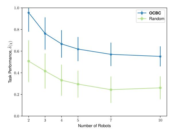
Figure 5.4: Effect of communication on task performance as a function of the number of simulated robots sharing a fixed amount of bandwidth. As team size increases, each robot has less opportunities to communicate, leading to decreased performance. Our method (*OCBC*), achieves better task performance compared to a randomized baseline method.
