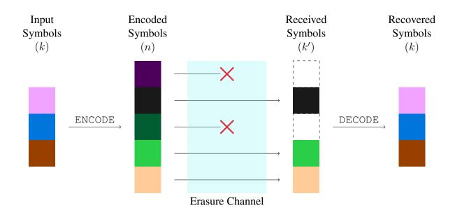
Figure 2.1: Illustration of erasure codes and their application to the erasure channel. k input symbols are encoded to produce the n symbols of the code word. These symbols are transmitted across the erasure channel, at which time some portion of the symbols may be erased. As long as a sufficient number k' of symbols are received, the original input message can be recovered.
