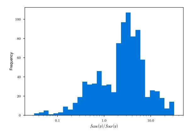
Figure 4.2: Frequency of relative likelihood of the kernel density estimation (KDE) and extended Kalman filter (EKF) distributions given samples collected from a real-world robotic network (see Section 4.5.1). We observe that for 82 percent of the samples, the KDEbased approach yielded a distribution of higher likelihood than the EKF-based approach of Section 3.4.2.
