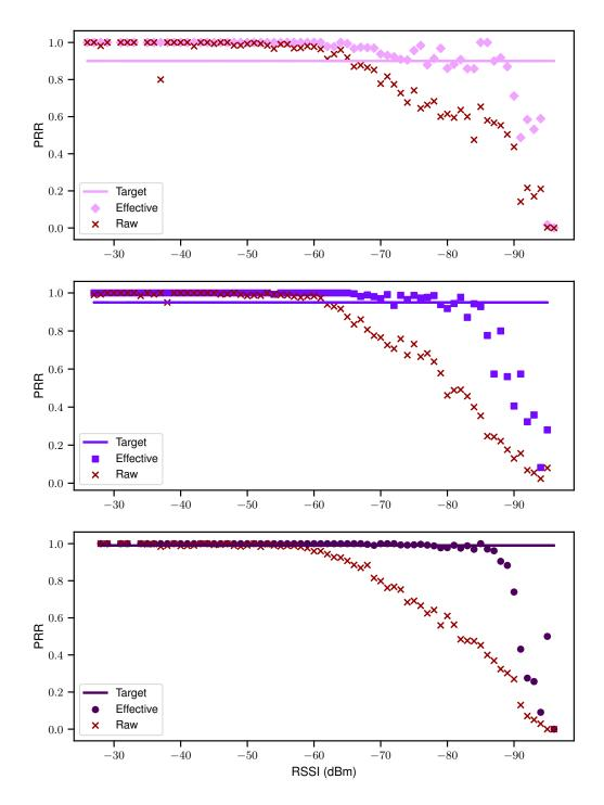
Figure 3.3: Effective packet reception ratio (PRR) achieved by Adaptive Erasure Coding (AEC) for varying target performance levels. The raw PRR declines as link quality decreases, but AEC is able to track a target effective PRR level. See Figure 3.4 for information on overhead levels required to achieve these improvements.
