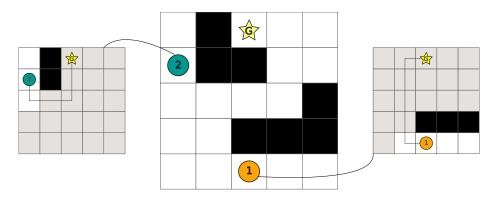
Figure 5.1: An example problem in which multiple robots independently navigate through an unknown environment. All robots try to reach the goal as quickly as possible; team reward depends on the total time taken by all robots. A robot observes the occupancy of adjacent cells as it moves through its environment. The robot can communicate these observations to its teammates to help them complete the task more quickly.
