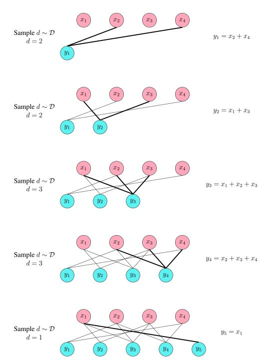
Figure 2.5: Tanner graph illustration of the fountain code encoding process. Input symbols  $x_1, \ldots, x_4$  are used to produce encoded symbols  $y_1, \ldots, y_5$ . For each encoded symbol, a degree d is sampled from the degree distribution  $\mathcal{D}$ . Then, d input symbols are sampled uniformly at random; the XOR of these input symbols is the encoded symbol.
