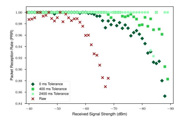
Figure 3.6: Close-up view of packet reception ratio (PRR) data from Figure 3.5. Increasing the amount of latency tolerance leads to a higher effective PRR.
