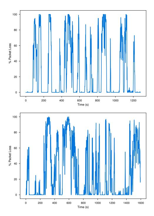
Figure 4.3: Time-series data of packet loss rates taken from mobile robotic network traces in indoor (*top*) and outdoor (*bottom*) environments. Note the frequent and rapid fluctuations in loss rates as well as the outages and near outages that occur. In total, the two traces comprise nearly 50 minutes of real-world network data.
