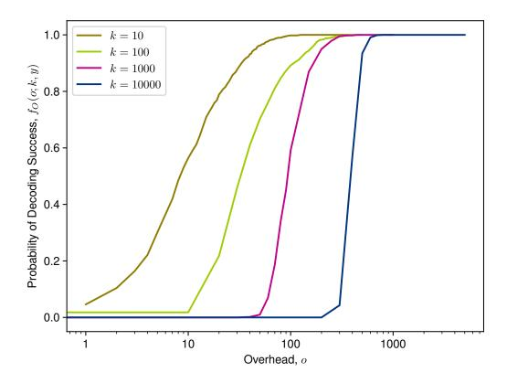
Figure 4.1: Decoding probability at varying levels of overhead for online codes [56]. The decoding probability of online codes is parameterized by the number of data symbols, k. For online codes, the decoding probability is independent of the packet reception ratio (PRR) y.
