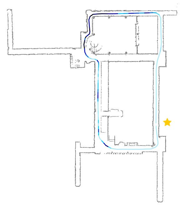
Figure 1.1: Visualization of instantaneous packet loss rates measured along a mobile robot's trajectory through an office building, with communication occurring between the robot and a stationary node (gold star). Darker colors indicate higher packet loss. We observe that the mobile robot experiences significant packet loss events as it travels through its environment and that the instantaneous packet loss rate can change rapidly.
