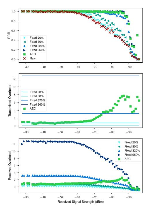
Figure 3.7: Comparison of Adaptive Erasure Coding (AEC) to a fixed erasure coding system similar to Google's Quick UDP Internet Connections (QUIC) [74]. The adaptive system yields effective PRR performance similar to the highest fixed method while using only a small fraction of the overhead.
