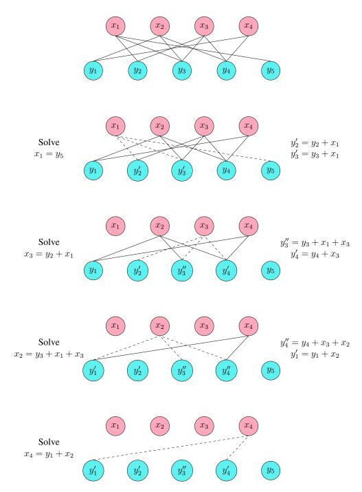
Figure 2.7: Tanner graph illustration of the fountain code decoding process. Encoded symbols of degree one are used to solve for input symbols. Any connections between the solved input symbols and encoded symbols are removed from the graph. This process repeats until all input symbols have been solved for.
