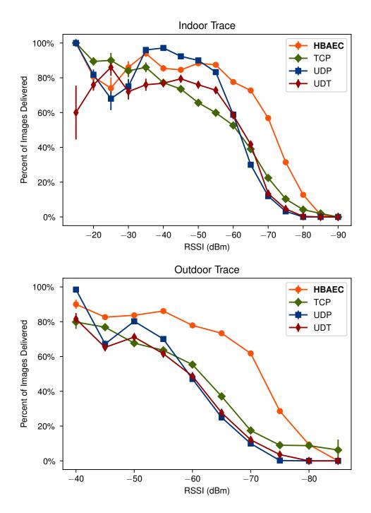
Figure 4.5: Image delivery performance of Figure 4.4 broken down by link quality. High Bandwidth Adaptive Erasure Coding (HBAEC) performs similarly to Transmission Control Protocol (TCP) in the high-quality link regime and outperforms it as link quality deteriorates.
