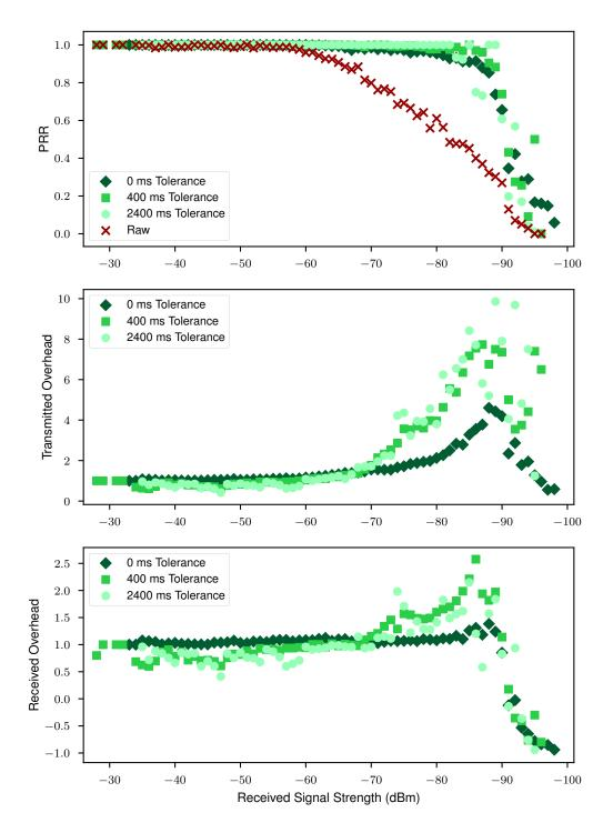
Figure 3.5: Packet reception ratio (PRR) and overhead results for an experiment with a fixed PRR target and variable latency tolerance. Increasing the amount of latency tolerance yields benefits in terms of effective PRR and overhead.
