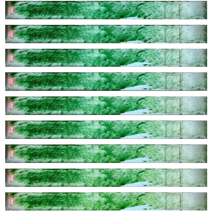
Figure 3.1: Trial 3W1 exhibited a very slight amount of sloughing. Resistance data in (a) show a drag increase of \Delta C_f \approx 85\text{--}110\% and only a moderate amount of hysteresis. Overhead pictures in (b) show the extent of fouling coverage. The top image in the series corresponds to the data at the beginning of the trial and the bottom images shows the fouling at the trial's end. The fifth image from the top was recorded at the maximum flow speed at the conclusion of the evolving leg of the trial (just before the stable portion began).
