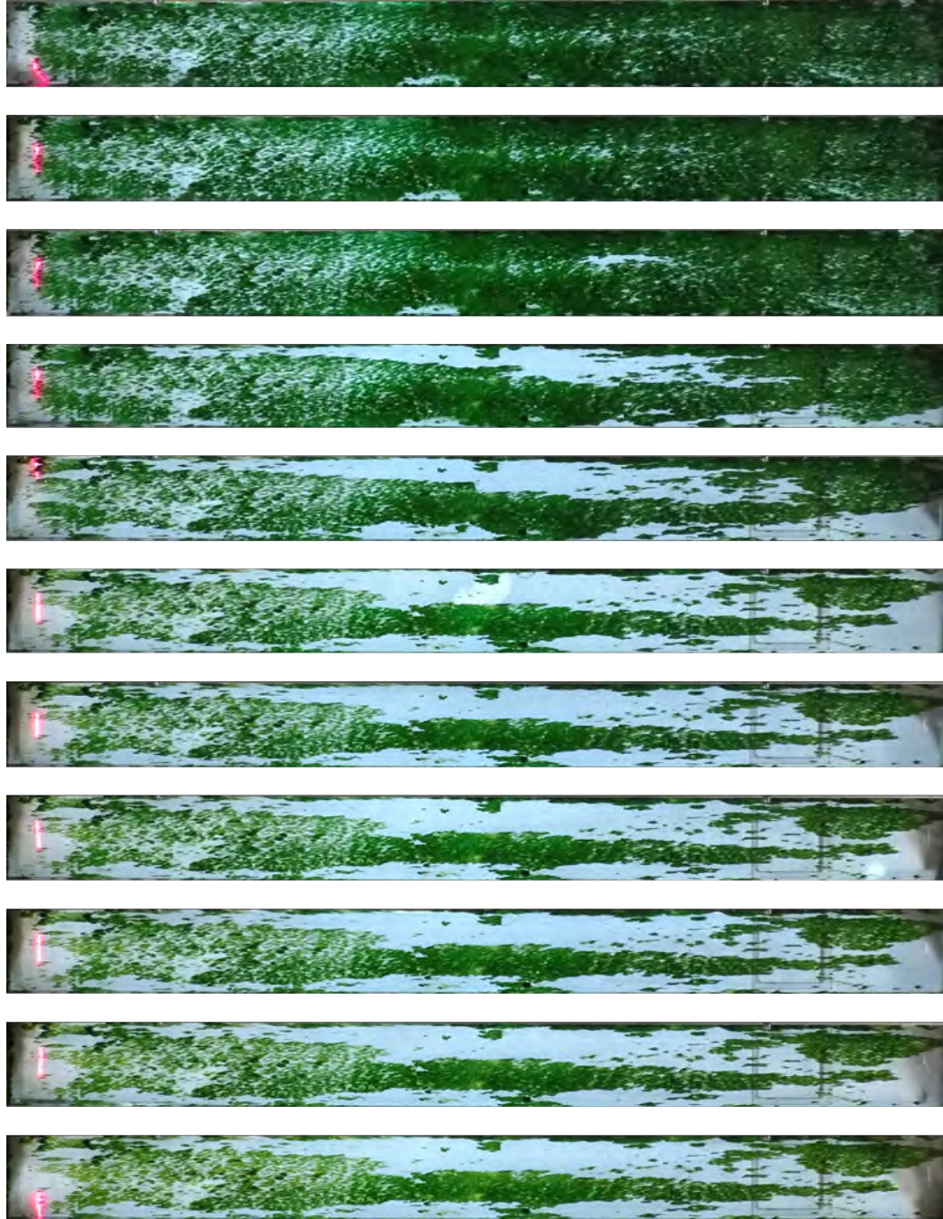
Figure 2.5: A series of images taken during biofilm Trial 5W2 shows the evolution of biofilm coverage due to bulk sloughing. For each trial, images were collected just before changing the flow rate using a GoPro Hero 5 black mounted above the SF3. Subsequent analysis of these images provides several parameters quantifying areal coverage.
