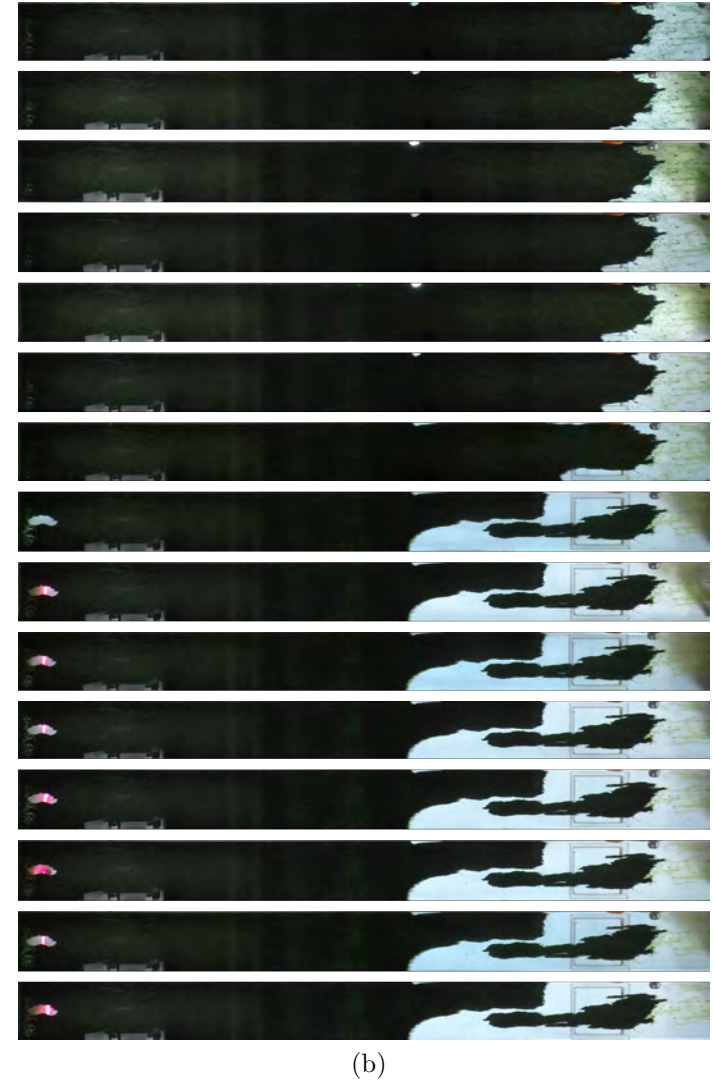
Figure 3.10: The biofilm layer was thickest in Trial 10W2 which also shows the greatest drag penalty, \Delta C_f , as seen in (a). Overhead photos (b) show that sloughing was limited to the downstream half of the panel. The eighth panel from the top in (b) corresponds to the maximum achieved flow speed.
