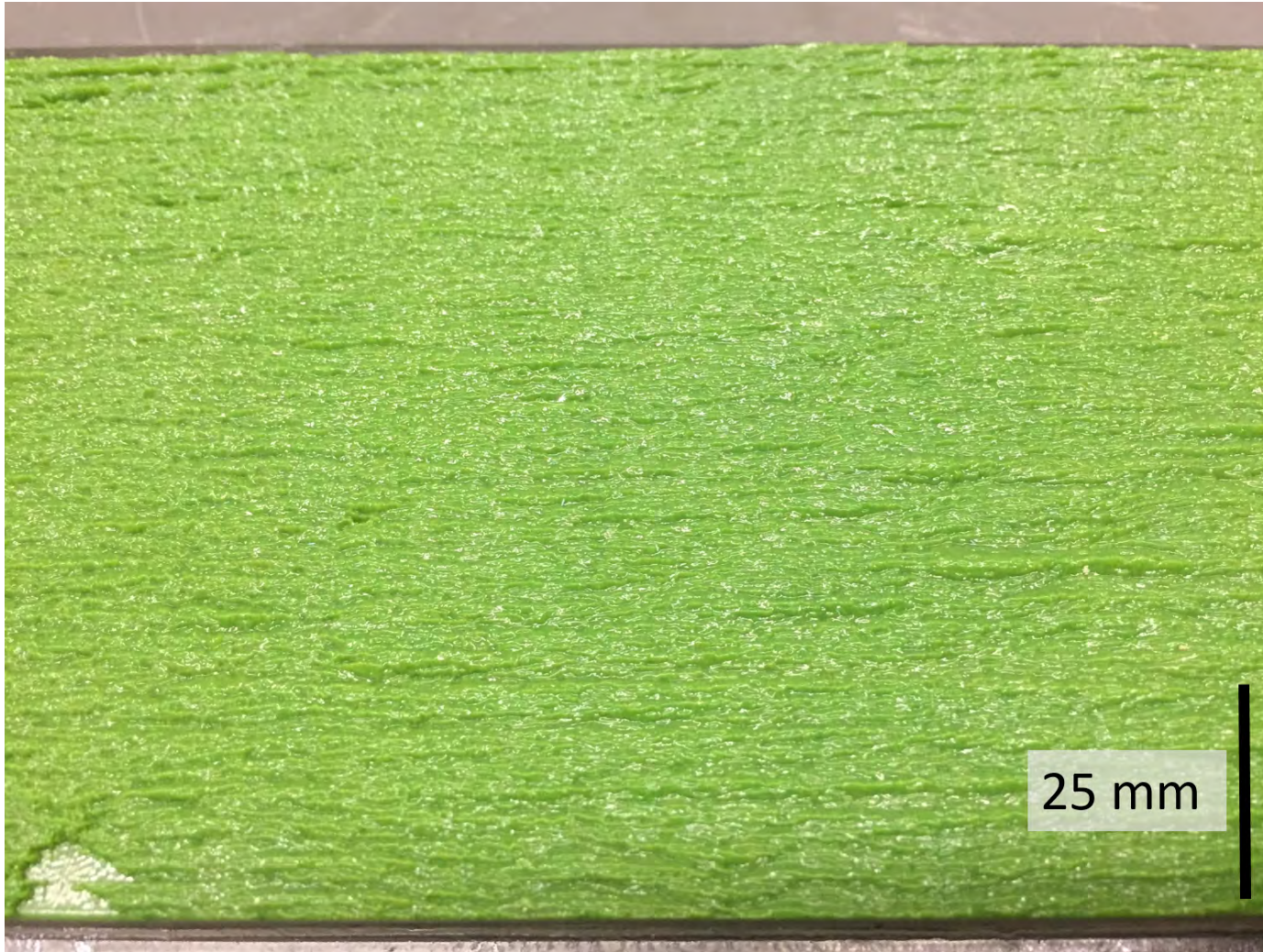
Figure 4.9: A portion of the rigid replica evaluated in Trial 10W2RR. Streamers were particularly elongated for this thickest of the biofilm layers. Note that the image shown here was taken at an angle to show better contrast between streamers which was not accounted for by the shown scale bar.
