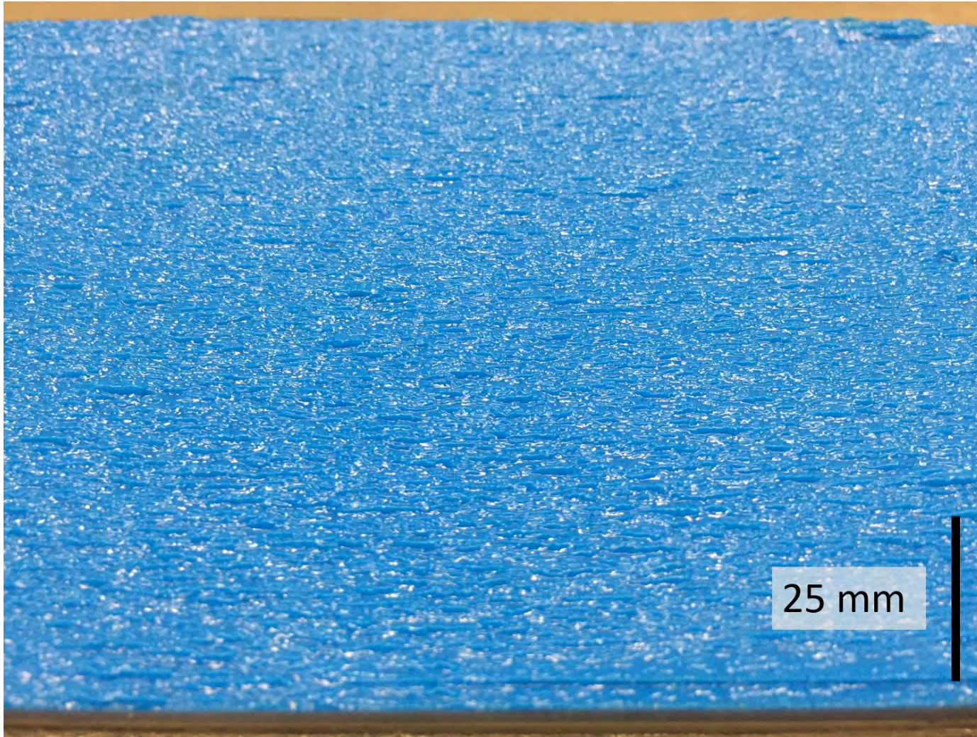
Figure 4.6: A close-up shows the texture of the rigid replica evaluated in Trial 5W3RRe. A dense patchwork of small streamers similar to those of Trial 5W1RR can be observed. Note that the image shown here was taken at an angle to show better contrast between streamers which was not accounted for by the shown scale bar.
