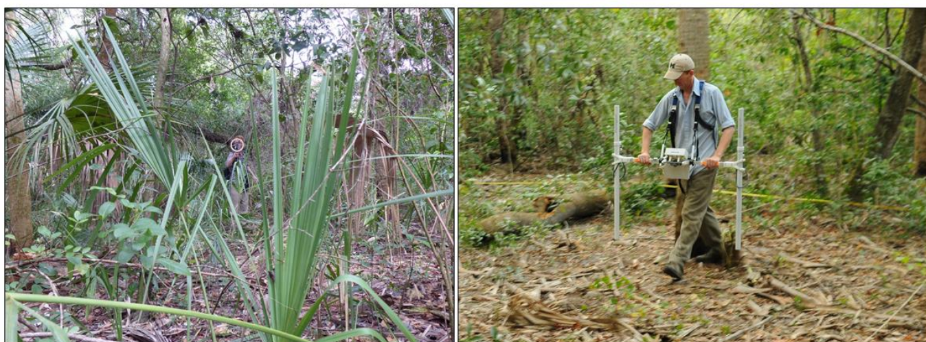
Figure 3.6 - Zeroing the susceptibility meter between readings under typical ground-cover conditions (left); conducting magnetometer survey in a cleared location (right)
