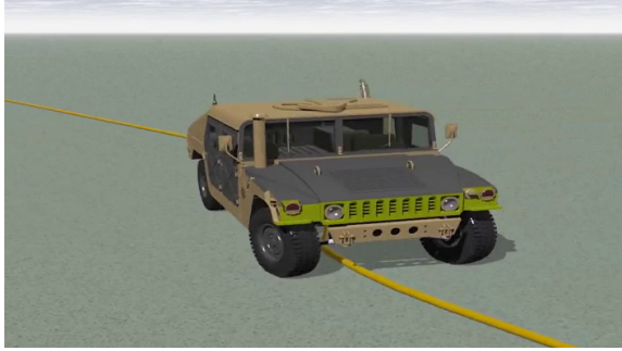
Figure 5.4: High-fidelity HMMWV model in Chrono used to model the plant [128].
