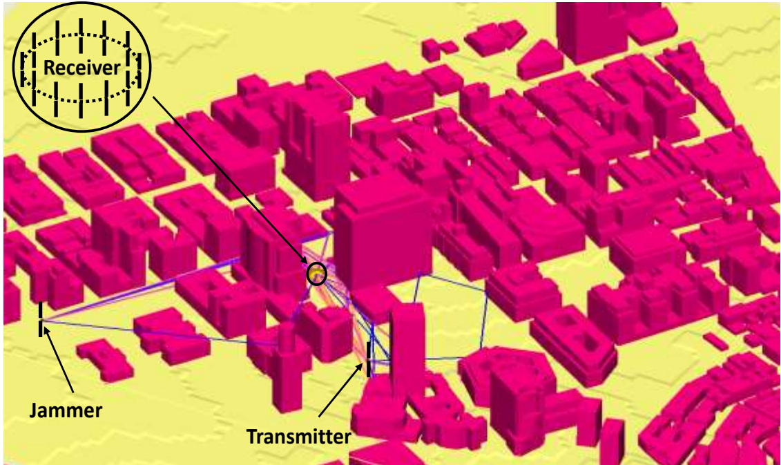
Figure 1-5: Ray tracing simulation results obtained by EMTerrano simulator for a scenario in Downtown Manhattan. A large number of rays arrive at the receiver array from both the communication transmitter and the jammer.
