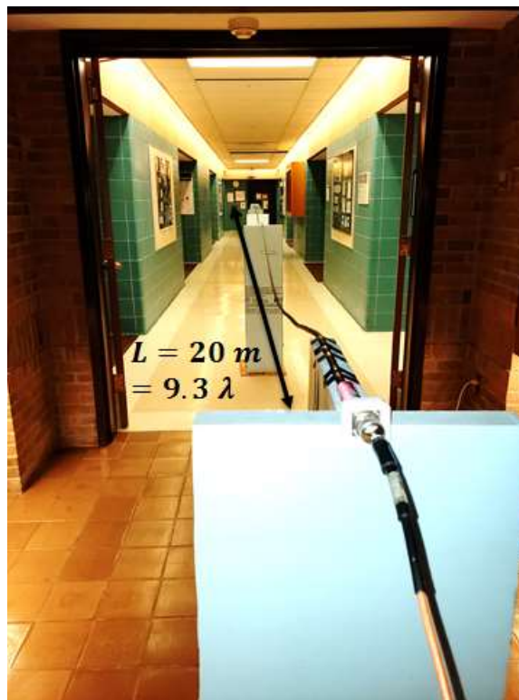
Figure 4-15. The experimental setup for testing the transducer. A 4AWG wire of length L = 9.3 \lambda = 20 m is used as the SCTL. The wire is terminated by the transducer at both ends. One transducer is excited by the network analyzer to measure the reflection coefficient. The transmitted power is P_t = 10 dBm. The receiving side is connected to the spectrum analyzer to measure the transmission loss.
