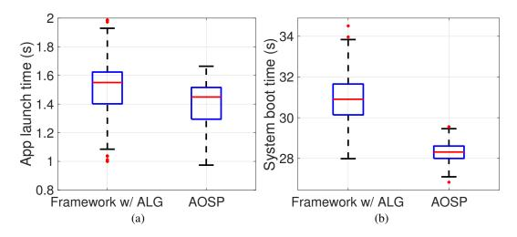
Figure 4.12: The comparison of application launch time and system boot between our framework and AOSP.
