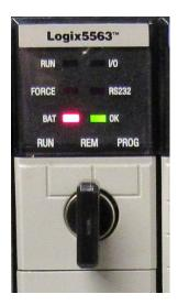
Figure 5.1: An Allen-Bradley ControlLogix 5563 PLC.
