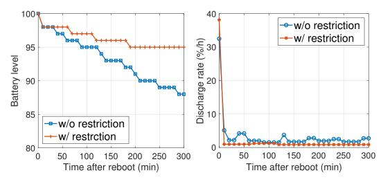
Figure 4.15: Battery life can be extended if diehard behaviors are restricted.
