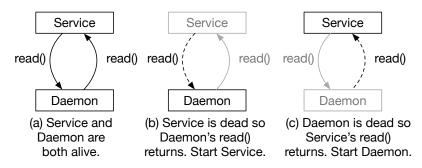
Figure 6.4: The Kaspersky application's service and daemon monitor each other through a Unix domain socket.
