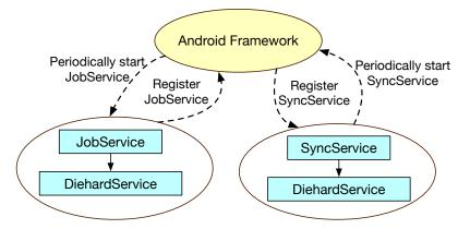
Figure 4.4: Partial ALG: cross-app ICC graph capturing scheduled task and account sync. Irrelevant ALG parts are omitted.
