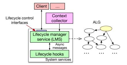
Figure 4.5: Overview of the framework. There could be multiple client apps that use the lifecycle control APIs.
