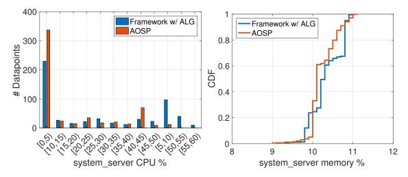
Figure 4.11: system\_server CPU and memory usage while repeatedly launching applications.
