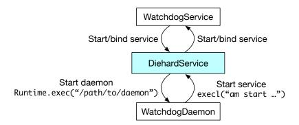
Figure 4.3: Partial ALG: intra-app ICC graph for an app having watchdog component. Irrelevant ALG parts are omitted.
