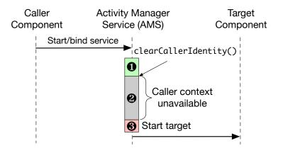
Figure 4.6: Hook placement options during service launching/binding ICC. The identity of the caller app is completely unavailable after the AMS calls clearCallerIdentity().
