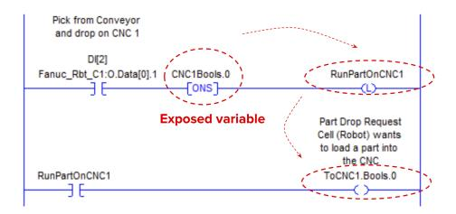
Figure 5.2: Example ladder logic with an exposed variable CNC1Bools. 0.
