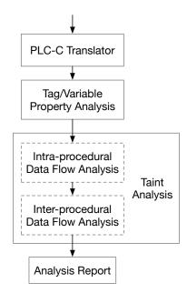
Figure 5.4: PLCAnalyzer analysis steps.
