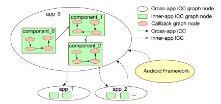
Figure 4.2: An ALG illustration. The Android framework is represented as a special node in the same level as apps. Edges have attributes that provide event contexts.
