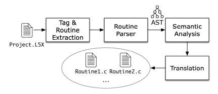
Figure 5.5: Translating PLC code into C.
