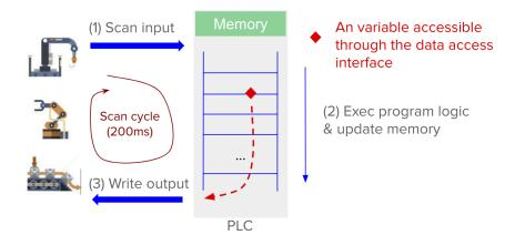
Figure 5.3: Safety-critical path illustration.
