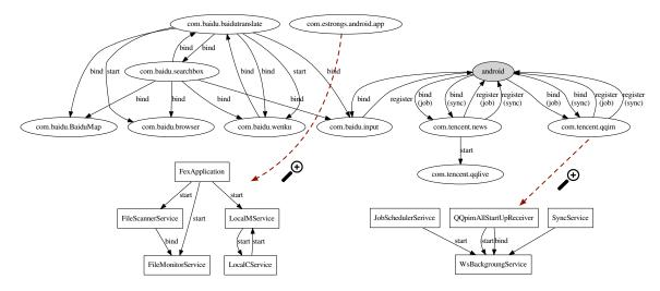
Figure 4.18: The topmost level (*i.e.*, cross-app ICC graph) of a real ALG visualized by Graphviz. com.estrongs.android.app and com.tencent.qqim are further inspected with one of their intra-app ICC graphs.
