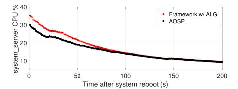
Figure 4.9: system\_server CPU usage after device reboot.
