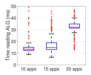
Figure 4.13: Difference in ALG reading time with different numbers of applications installed on the device.
