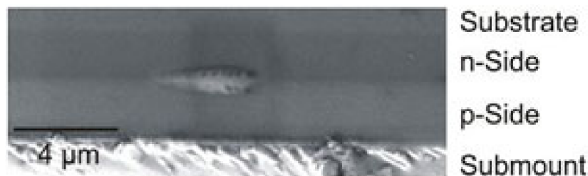
Figure 7.2.1 | Dark-line defects at the outcoupling facet observed under a microscope. Image courtesy of ref. [3].
