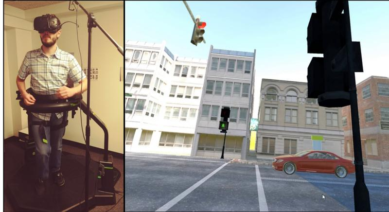
**Figure 2.** Virtual Reality setup for user study. The left side shows the user wearing the HTC Vive headset and walking on the omni-directional treadmill. The right side shows the virtual environment as seen by the participant.
