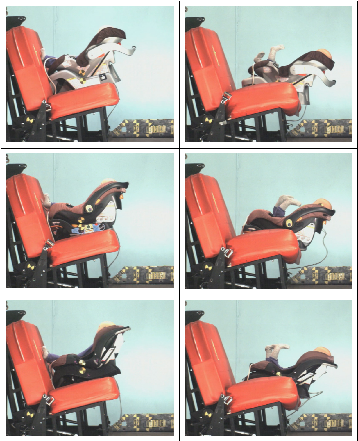
Figure 4. Time-zero and maximum rotation video frames for each test conducted with the CRABI-18.
