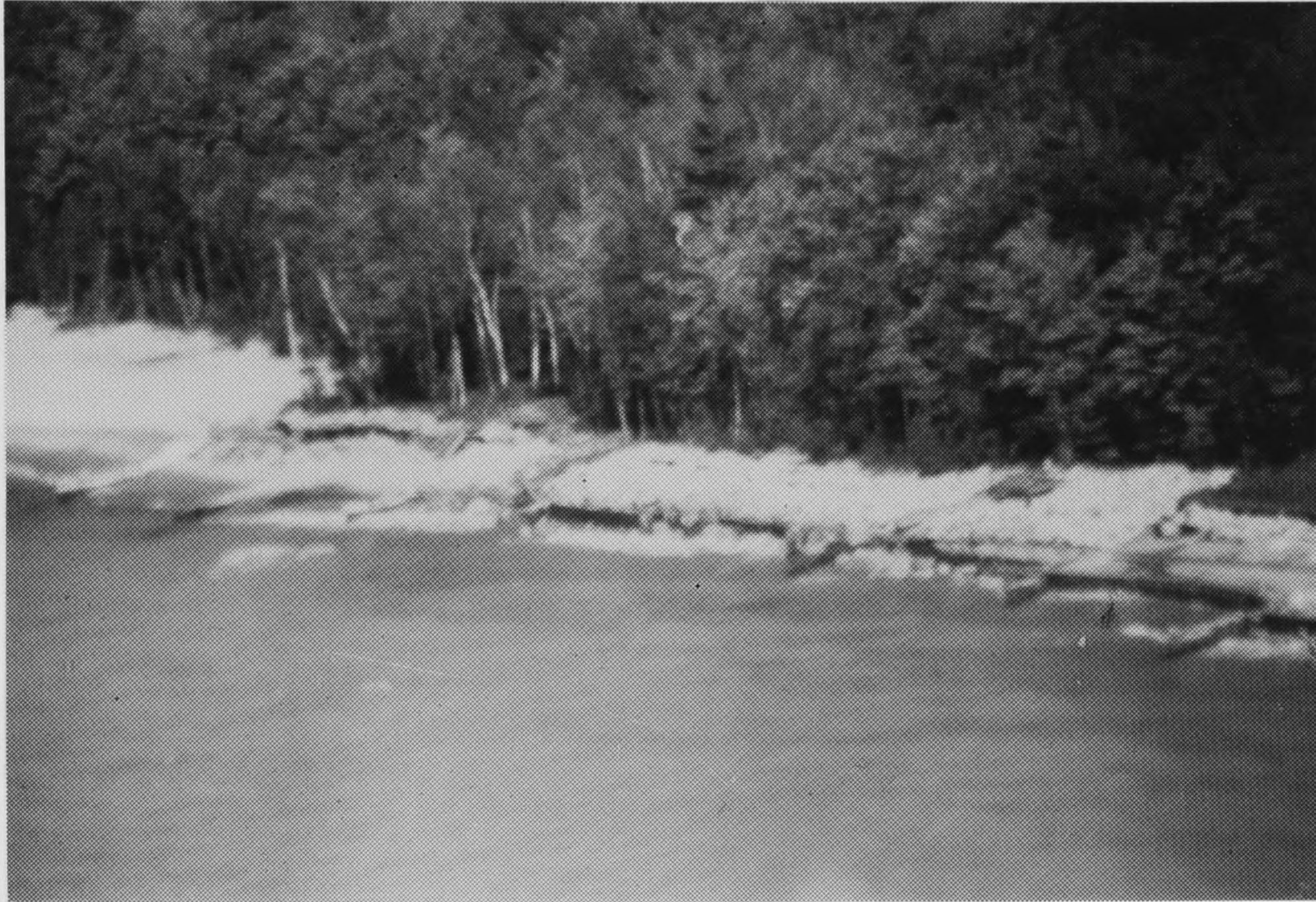
Figure B42. Site O: Aerial view of short revetment at north side of property. Recession of shoreline to north of revetment is visible at left center of photo.
