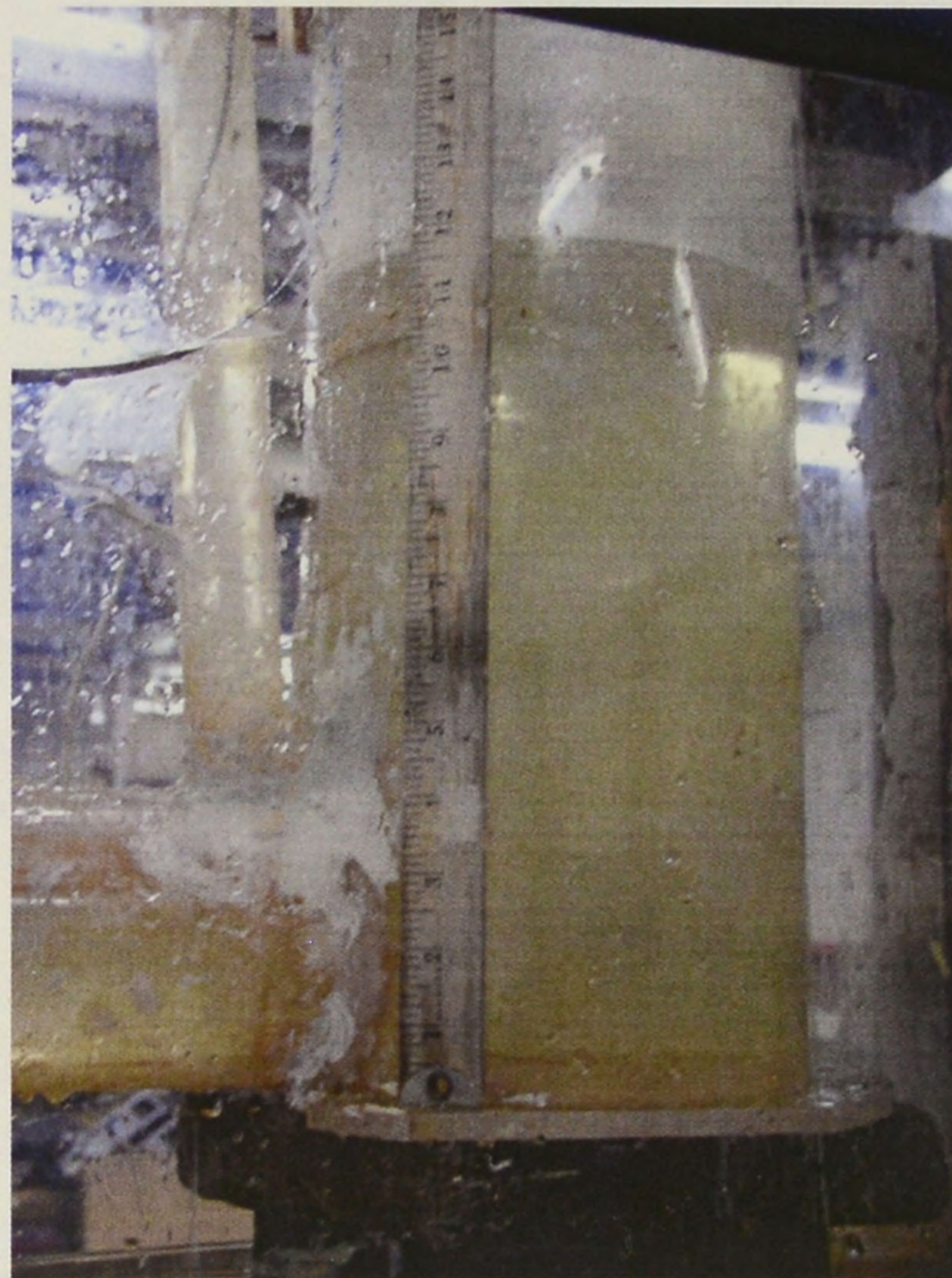
Figure 2.2: Photograph of the surge tank used in the experiments
