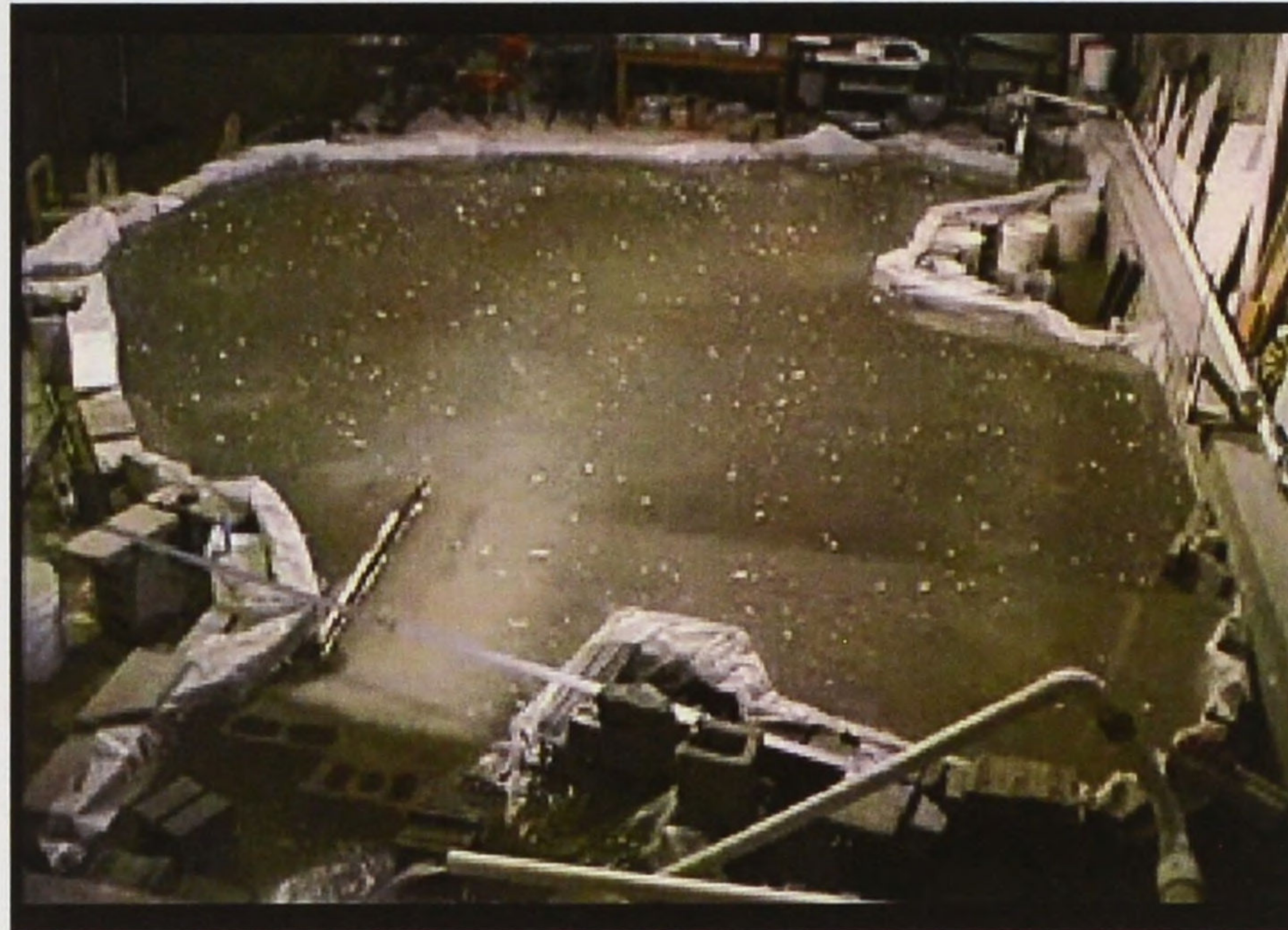
Figure 3 – Constructed Scale Model of Kalamazoo Lake (Including single arm seawall)
