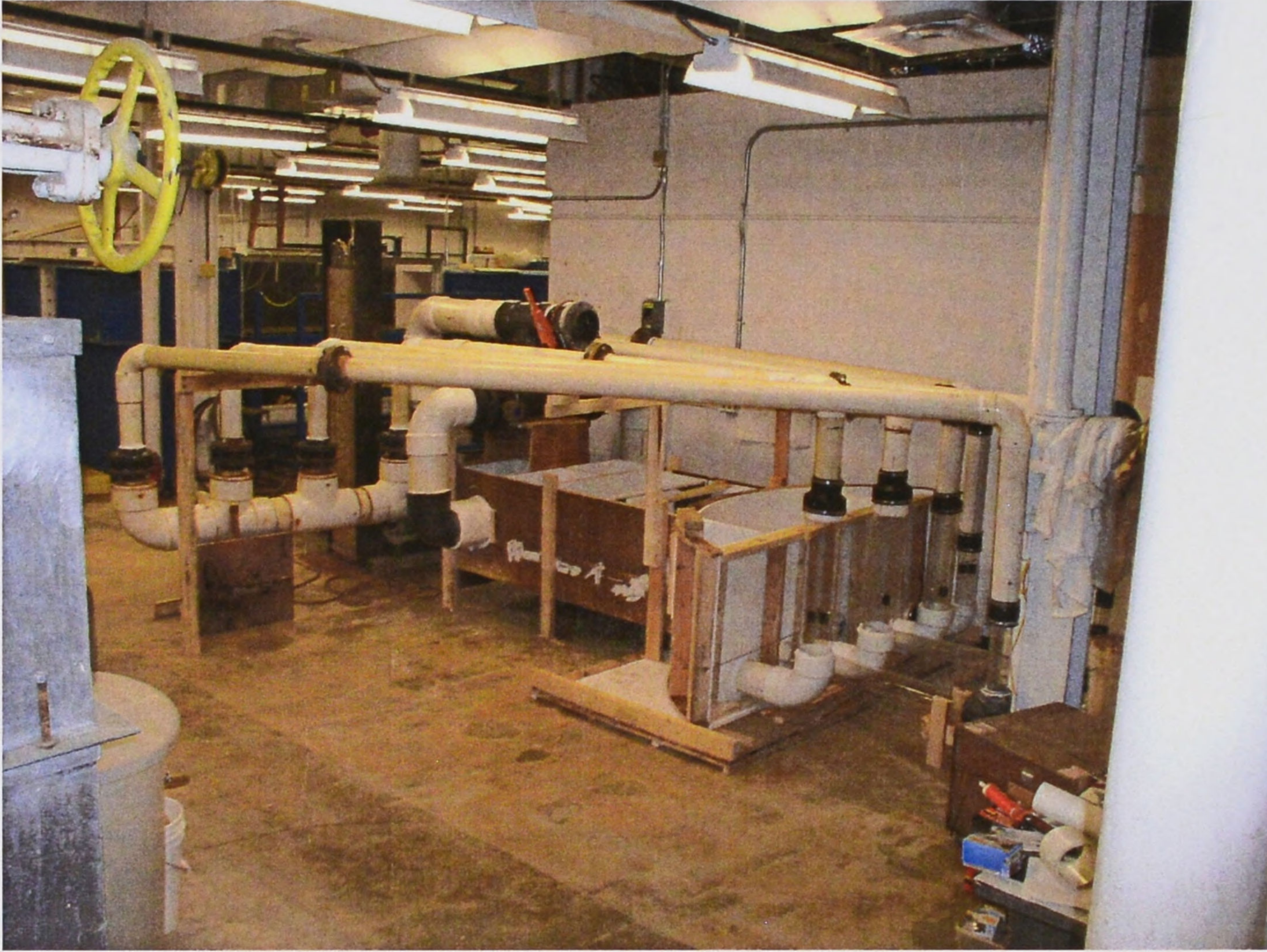
Figure 4. Wyandotte WWTP Influent Pump Station physical hydraulic model.
