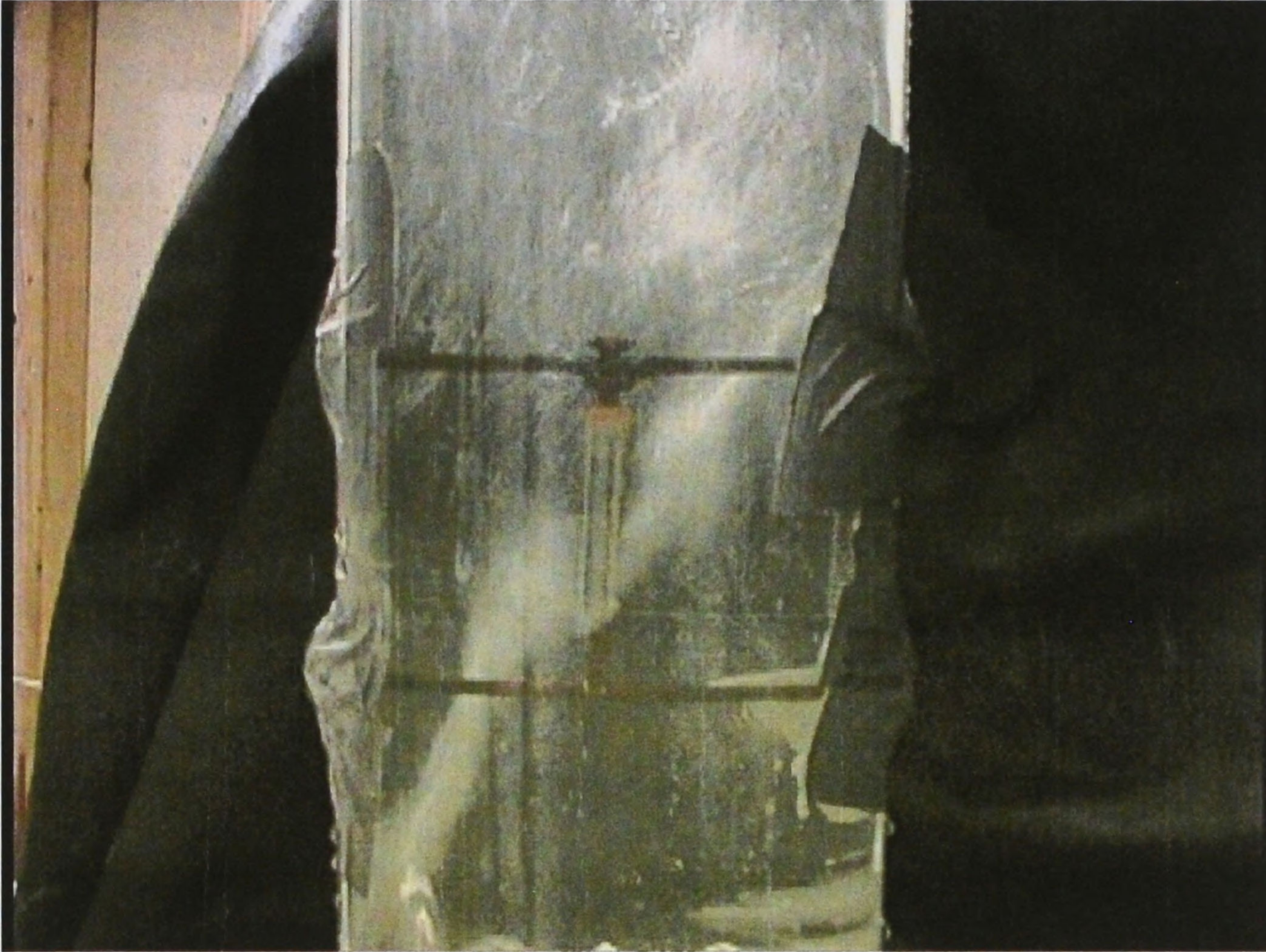
Figure 12. Air entrainment into Pump #5 for a low wet well level with Pumps # 2, 3, 5, and 6 in operation.
