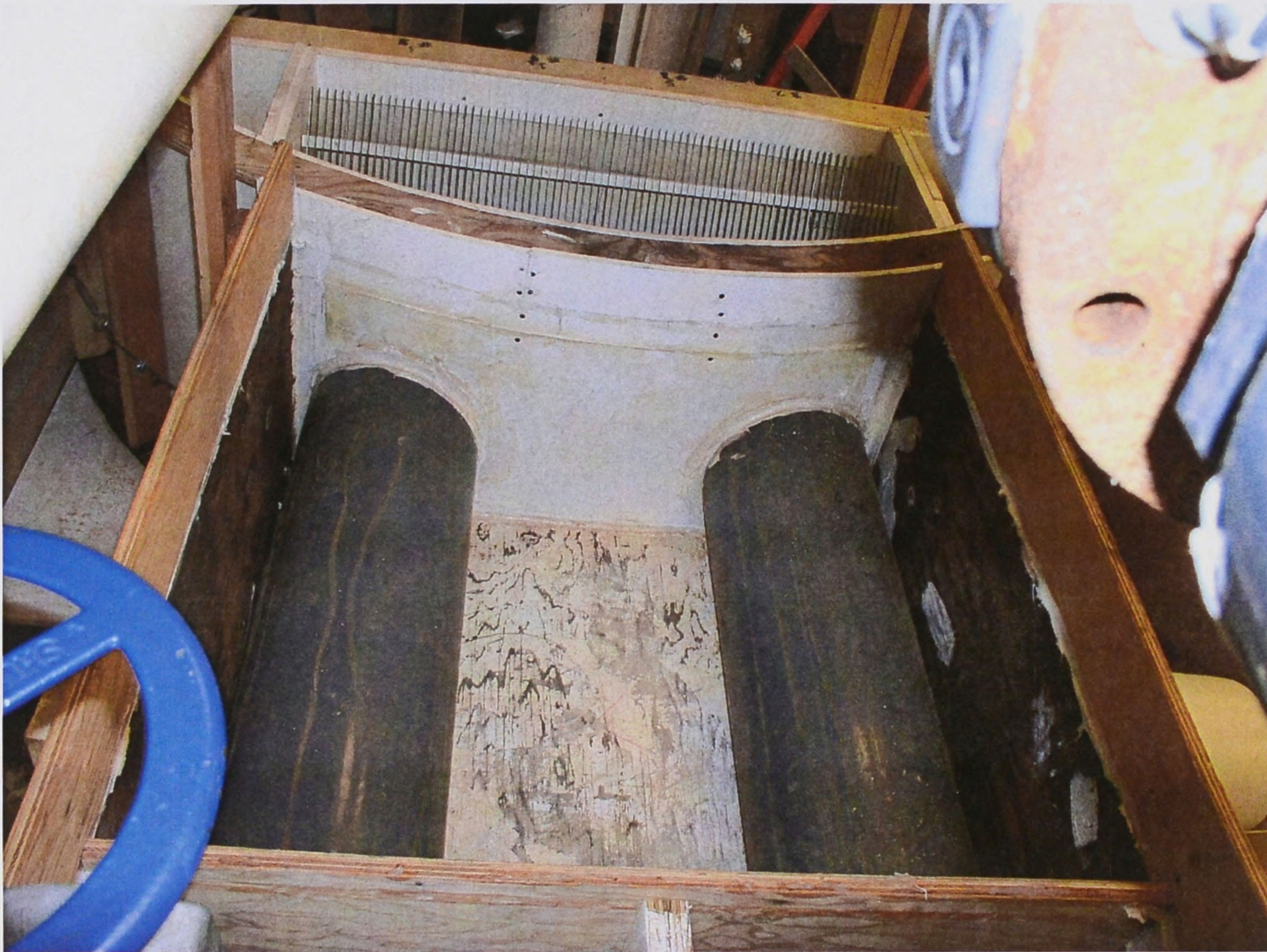
Figure 10. Model Modifications to represent “original” Inlet Conditions.
