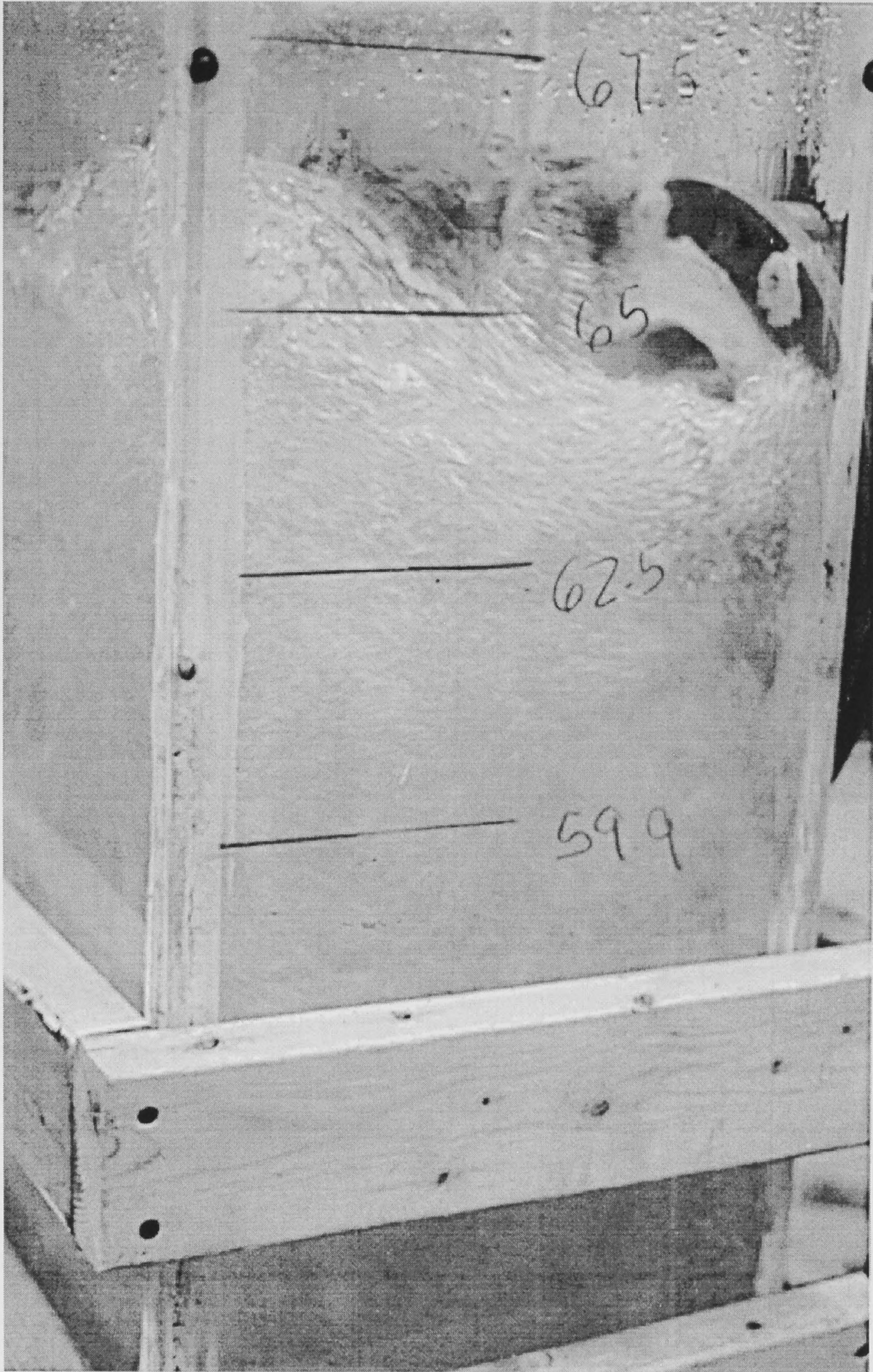
Figure 4a. Air Entrainment at Intermediate Water Level in East Drop Shaft.
