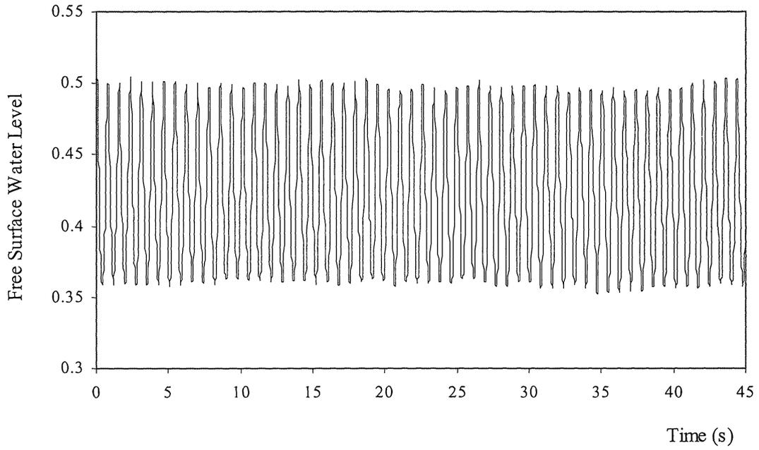
**Figure 10a. Typical Water Surface Displacement Record. ( $T = 6$  s,  $280^\circ$ )**
