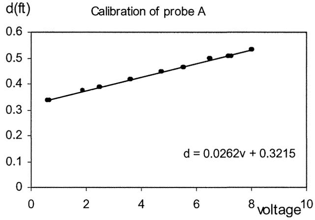
Figure A-1. Calibration Curve for Probe A
