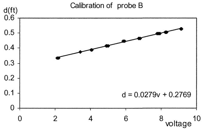
Figure A-2. Calibration Curve for Probe B
