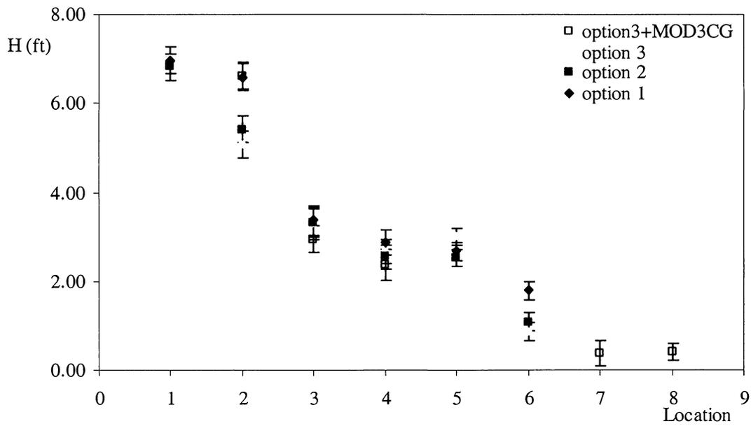
Figure 23. Comparison of the three proposed modifications for a wave period of  $T = 5s$  and an incoming wind angle of  $260^\circ$ .
