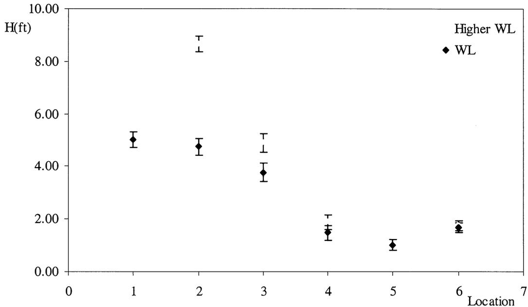
**Figure 37. Results for a 4 ft. increase in the free surface water level. Wave period of  $T = 7s$  and an incoming wind angle of  $260^\circ$ . Option 3.**
