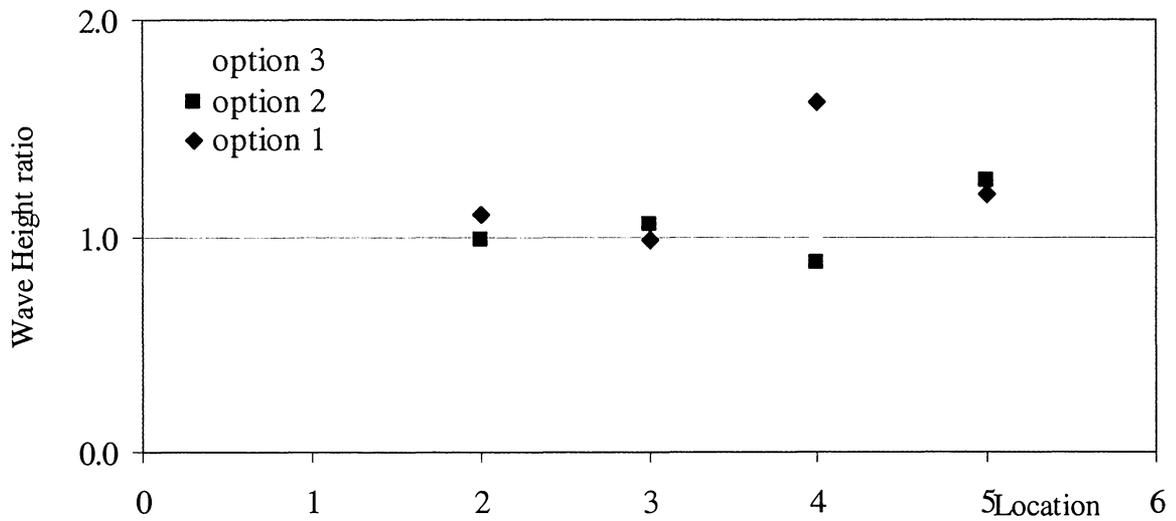
*Figure 39. Wave Height ratios for a free surface water level increase of 4 ft. Wave period of  $T = 7s$  and an incoming wave angle of  $260^\circ$ .*
