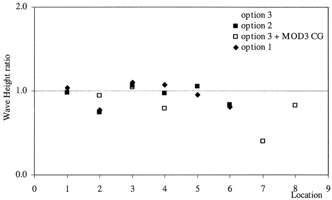
Figure 28. Wave Height Ratio comparison for a wave period of  $T = 6s$  and an incoming wave angle of  $280^\circ$ .
