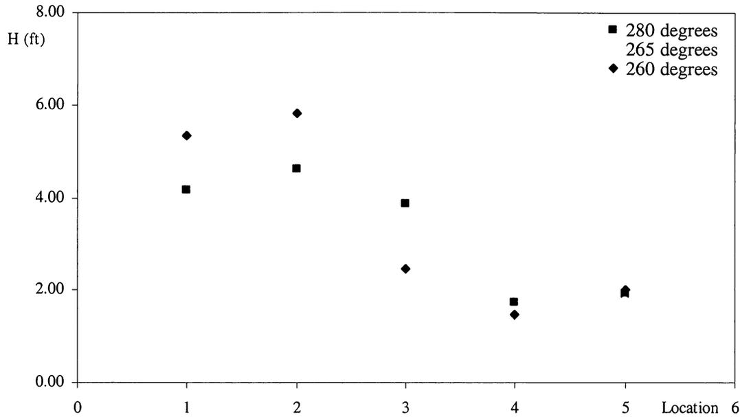
**Figure 19. Comparison of measured wave heights for three different incident wave directions.**
