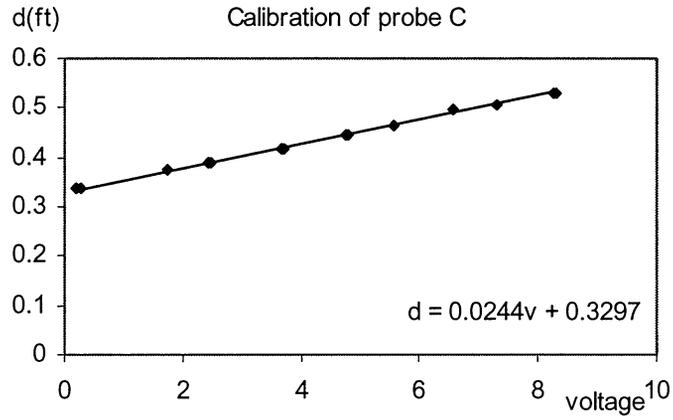
Figure A-2. Calibration Curve for Probe C
