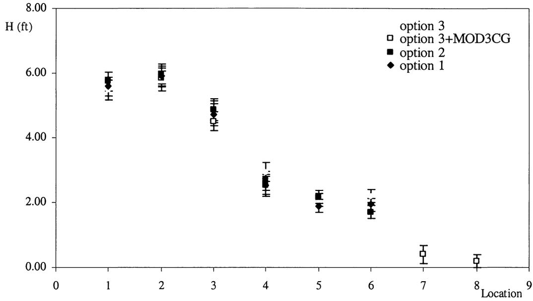
*Figure 20. Comparison of the three proposed modifications for a wave period of  $T = 5s$  and an incoming wind angle of  $280^\circ$ .*
