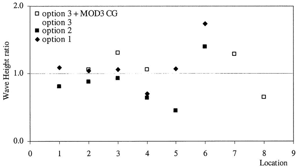
**Figure 31.** Wave Height Ratio comparison for a wave period of  $T = 7s$  and an incoming wave angle of  $260^\circ$ .
