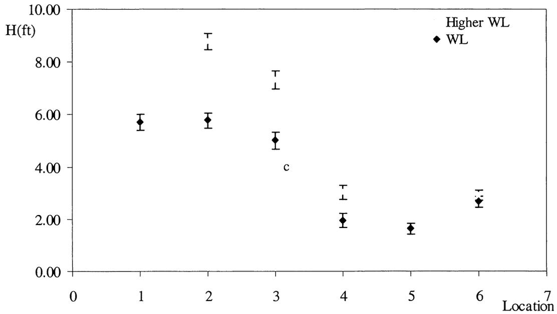
**Figure 34. Results for a 4 ft. increase in the free surface water level. Wave period of  $T = 6s$  and an incoming wind angle of  $280^\circ$ . Option 3.**
