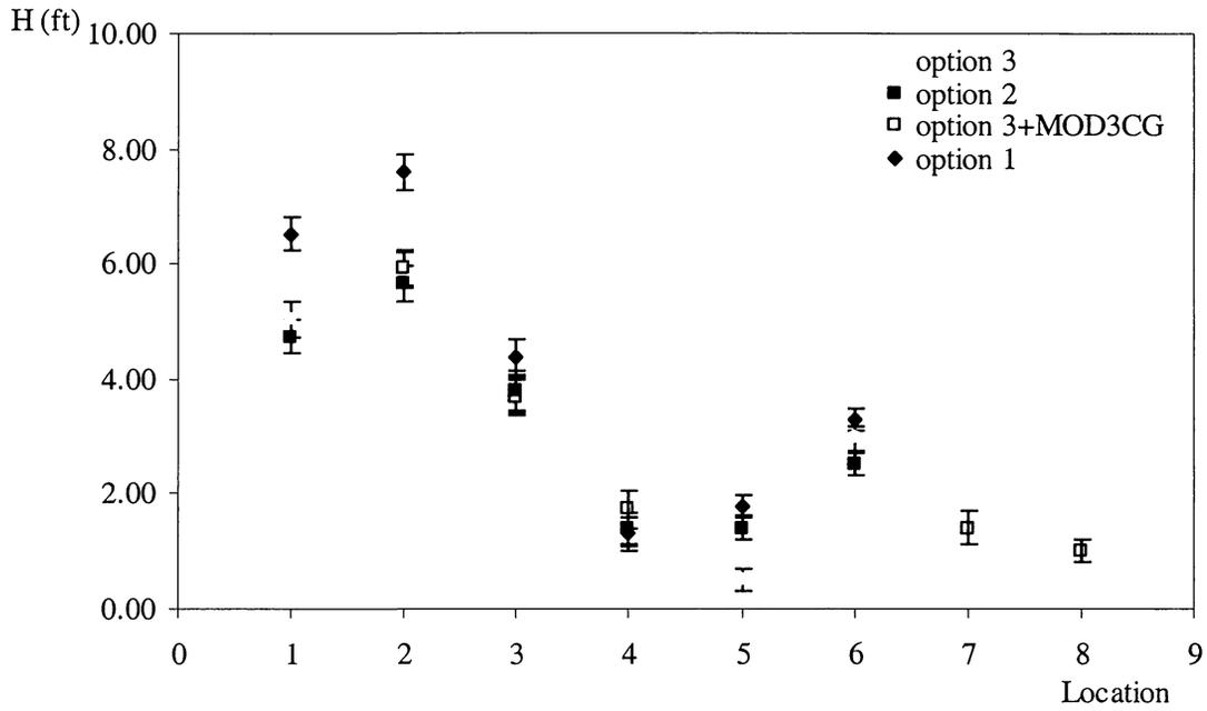
*Figure 24. Comparison of the three proposed modifications for a wave period of  $T = 6s$  and an incoming wind angle of  $260^\circ$ .*
