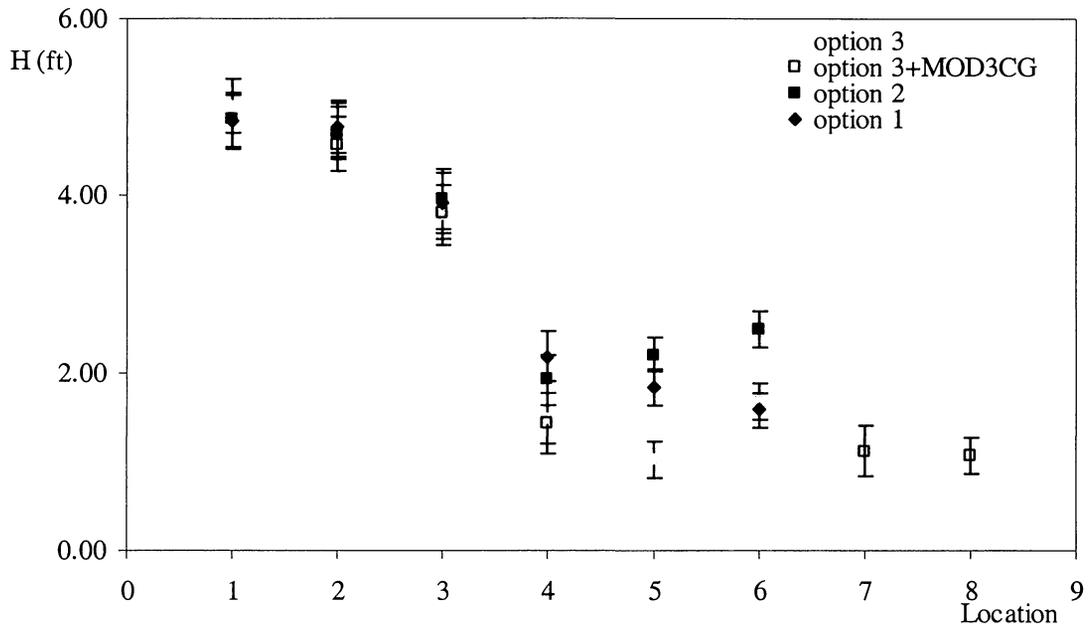
Figure 22. Comparison of the three proposed modifications for a wave period of  $T = 7s$  and an incoming wind angle of  $280^\circ$ .
