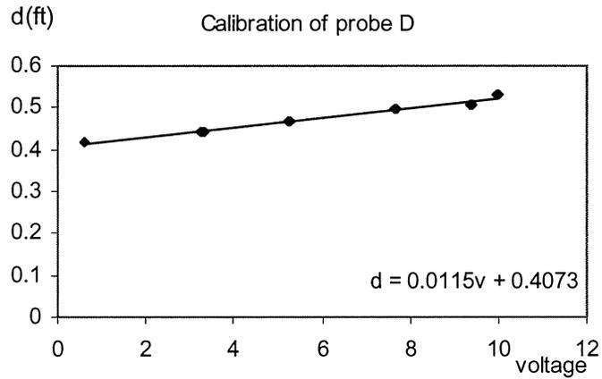
Figure A-3. Calibration Curve for Probe D
