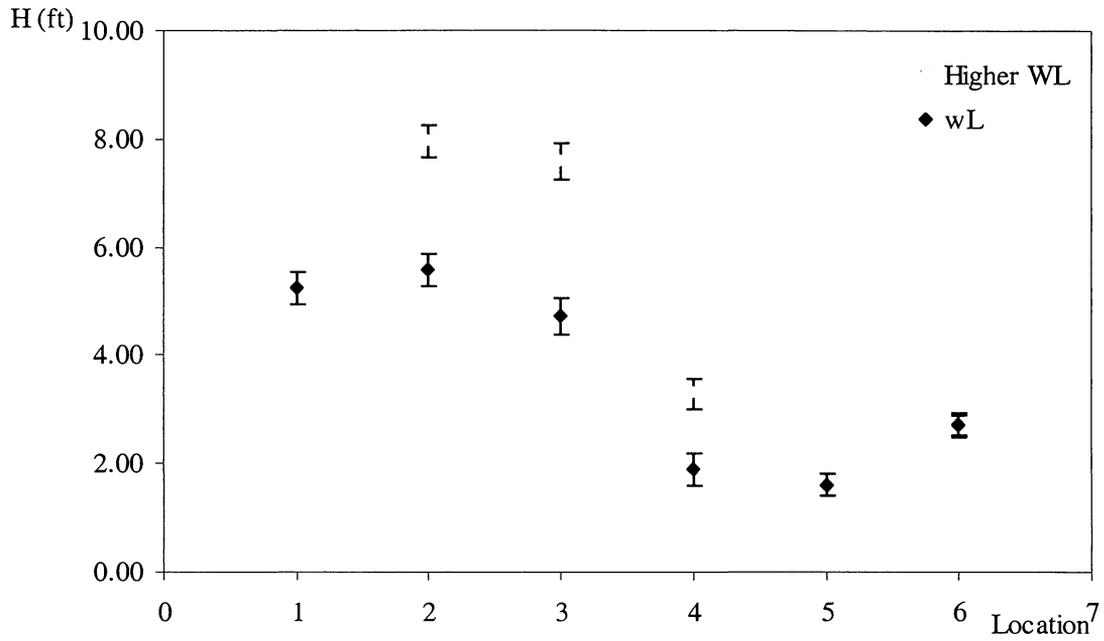
**Figure 33. Results for a 4 ft. increase in the free surface water level. Wave period of  $T = 6s$  and an incoming wind angle of  $280^\circ$ . Option 2.**
