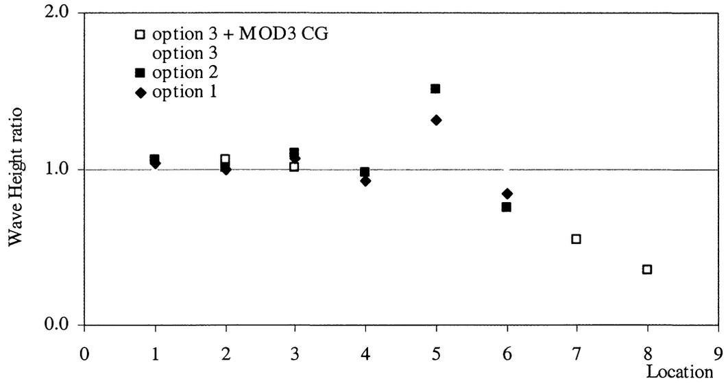
**Figure 26. Wave Height Ratio comparison for a wave period of  $T = 5s$  and an incoming wave angle of  $280^\circ$ .**
