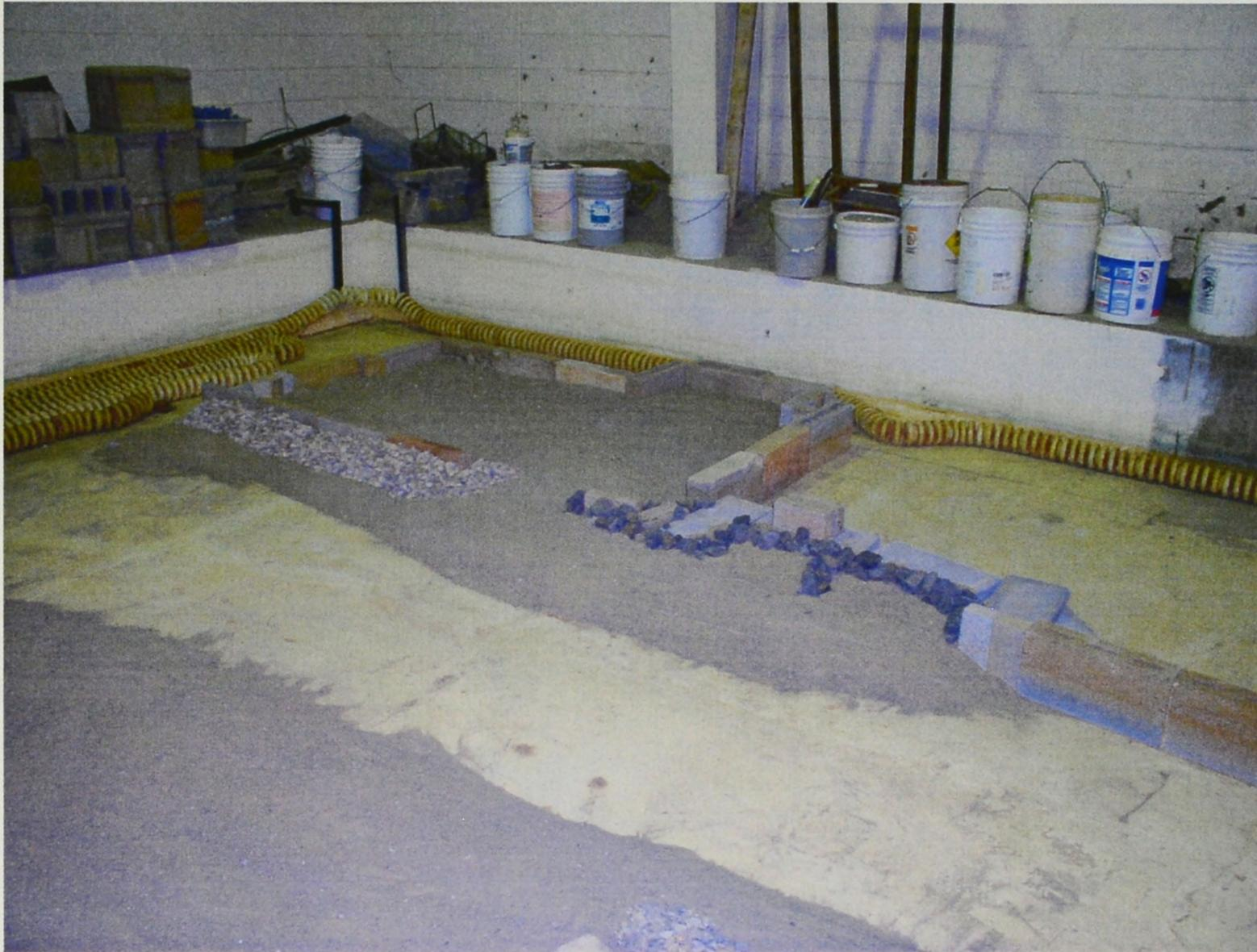
***Figure 11. Harbor bathymetry reproduced in the model with concrete blocks and sand, looking towards Waterfront Marina.***
