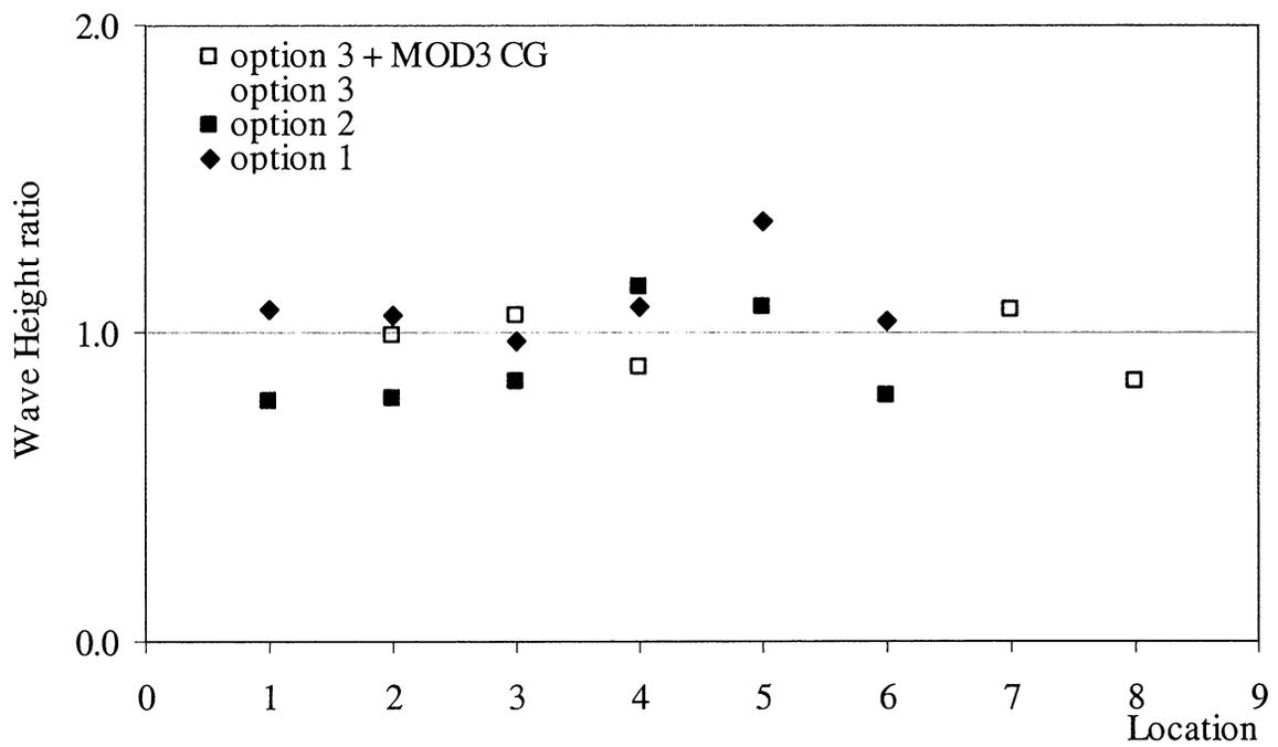
Figure 29. Wave Height Ratio comparison for a wave period of  $T = 6s$  and an incoming wave angle of  $260^\circ$ .
