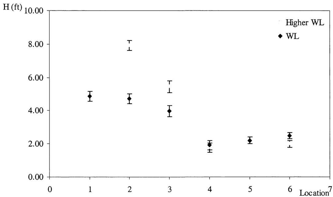
**Figure 36. Results for a 4 ft. increase in the free surface water level. Wave period of  $T = 7s$  and an incoming wind angle of  $260^\circ$ . Option 2.**
