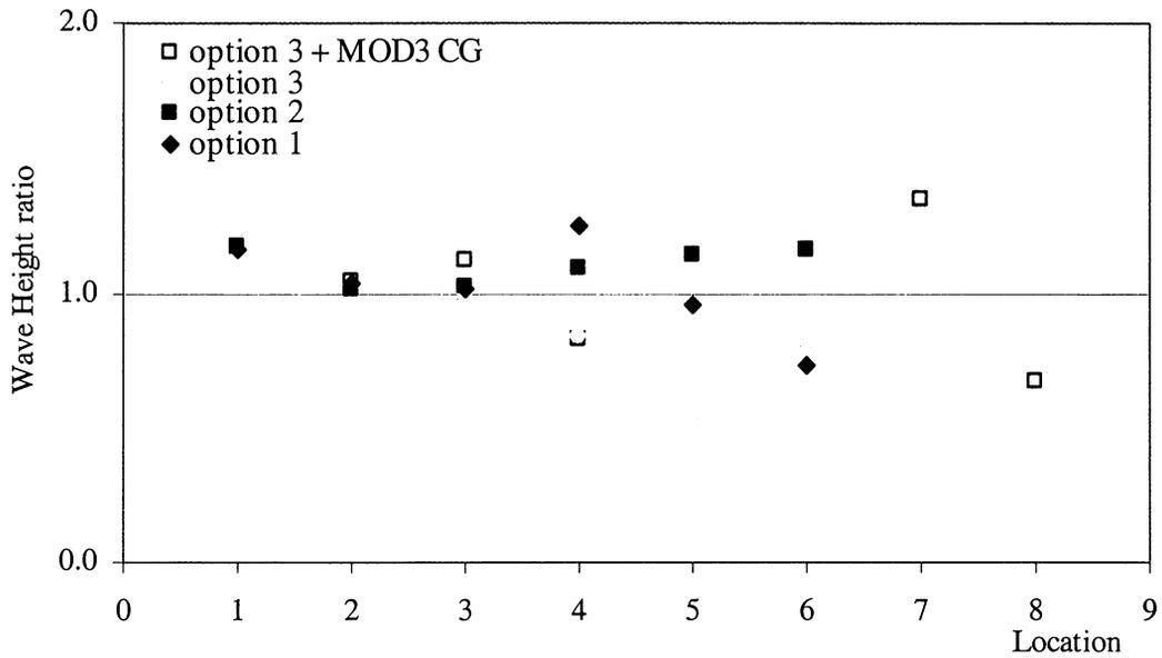
**Figure 30.** Wave Height Ratio comparison for a wave period of  $T = 7s$  and an incoming wave angle of  $280^\circ$ .
