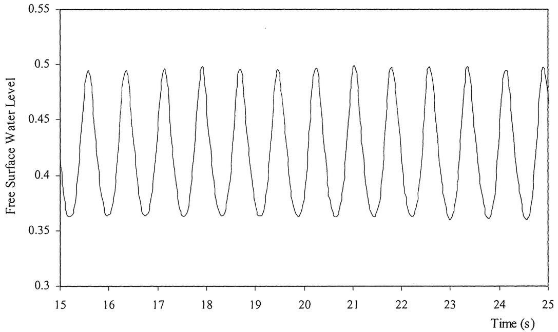
**Figure 10b. Sample of a Water Surface Displacement Record. ( $T = 6$  s,  $280^\circ$ )**
