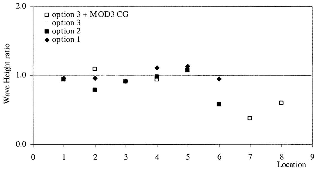
**Figure 27. Wave Height Ratio comparison for a wave period of  $T = 5s$  and an incoming wave angle of  $260^\circ$ .**
