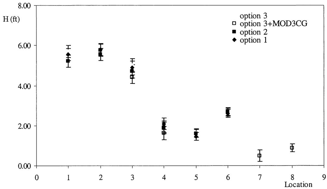
*Figure 21. Comparison of the three proposed modifications for a wave period of  $T = 6s$  and an incoming wind angle of  $280^\circ$ .*
