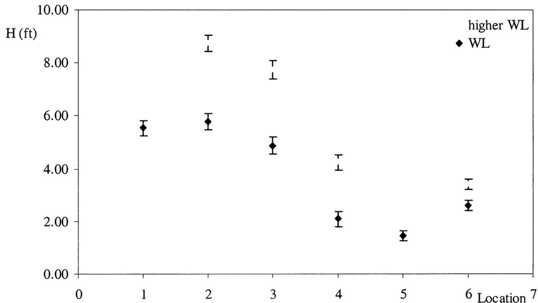
**Figure 32. Results for a 4 ft. increase in the free surface water level. Wave period of  $T = 6s$  and an incoming wind angle of  $280^\circ$ . Option 1.**
