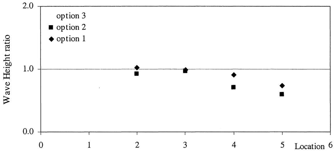
*Figure 38. Wave Height ratios for a free surface water level increase of 4 ft. Wave period of  $T = 6s$  and an incoming wave angle of  $280^\circ$ .*
