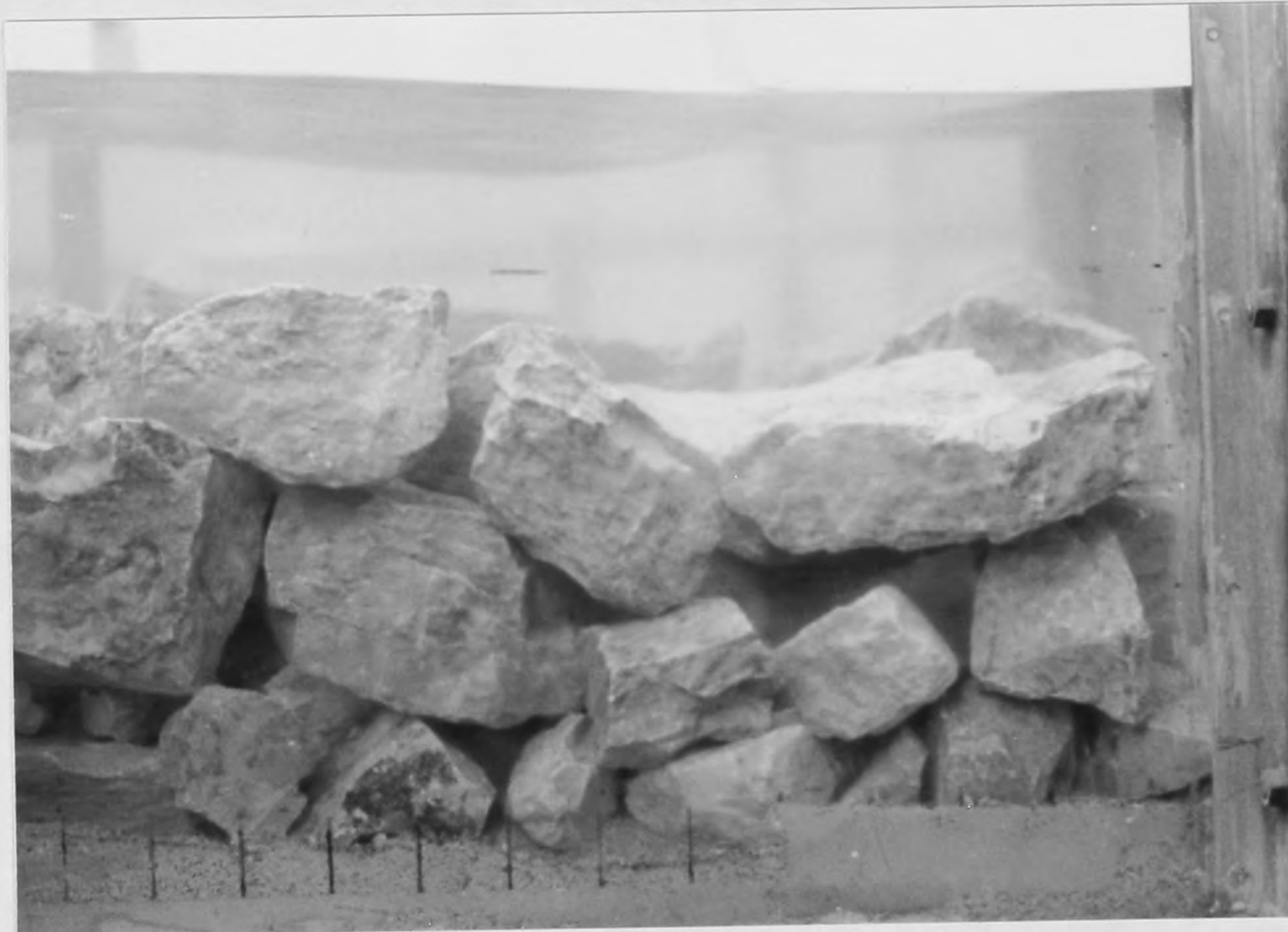
FIG. 5. Test Section During the Experiment (Showing Water Surface Level Decline in the Direction of Flow)
