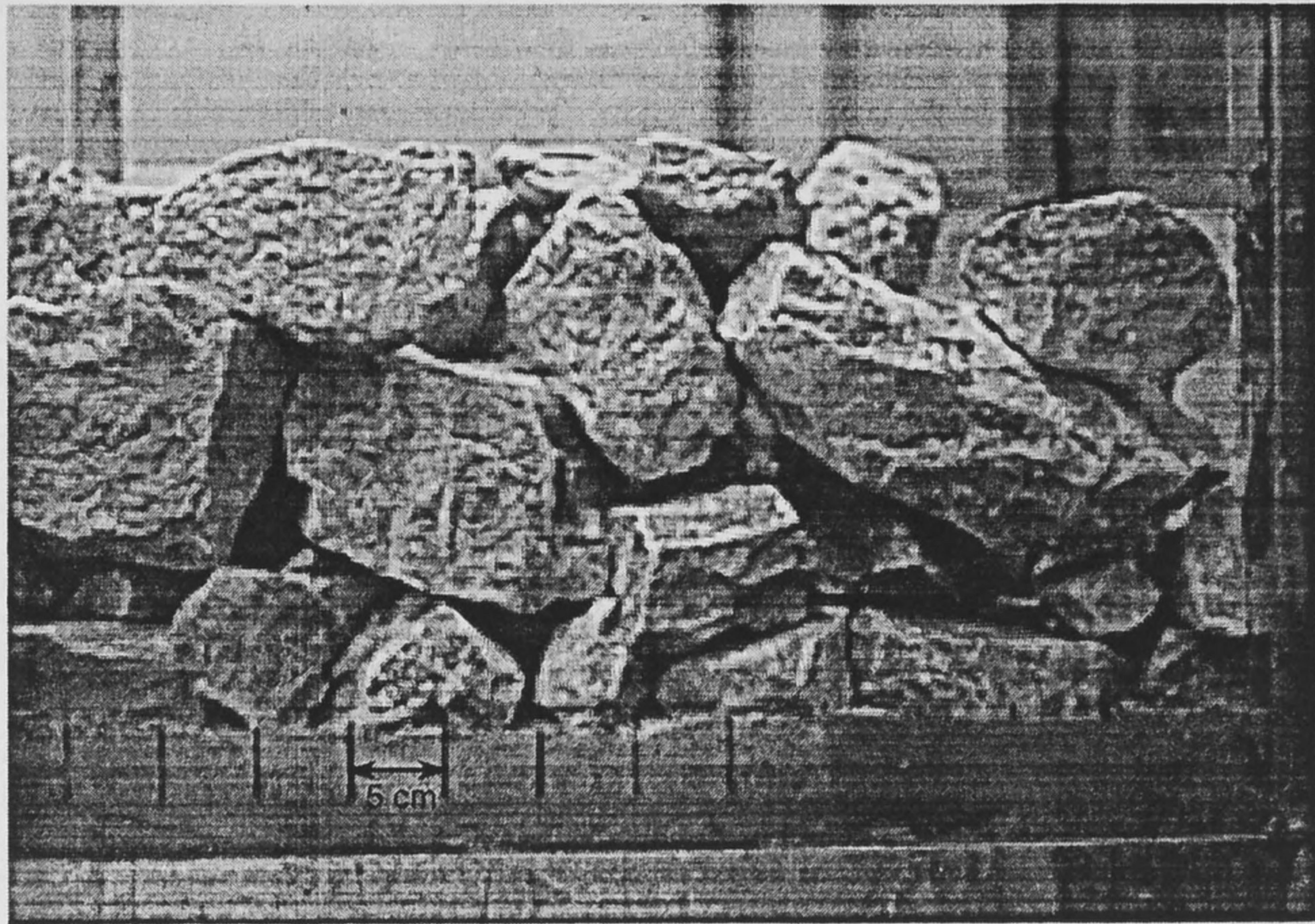
FIGURE 4c. Completed test section with final layer of 4-8 inch dolomite.
