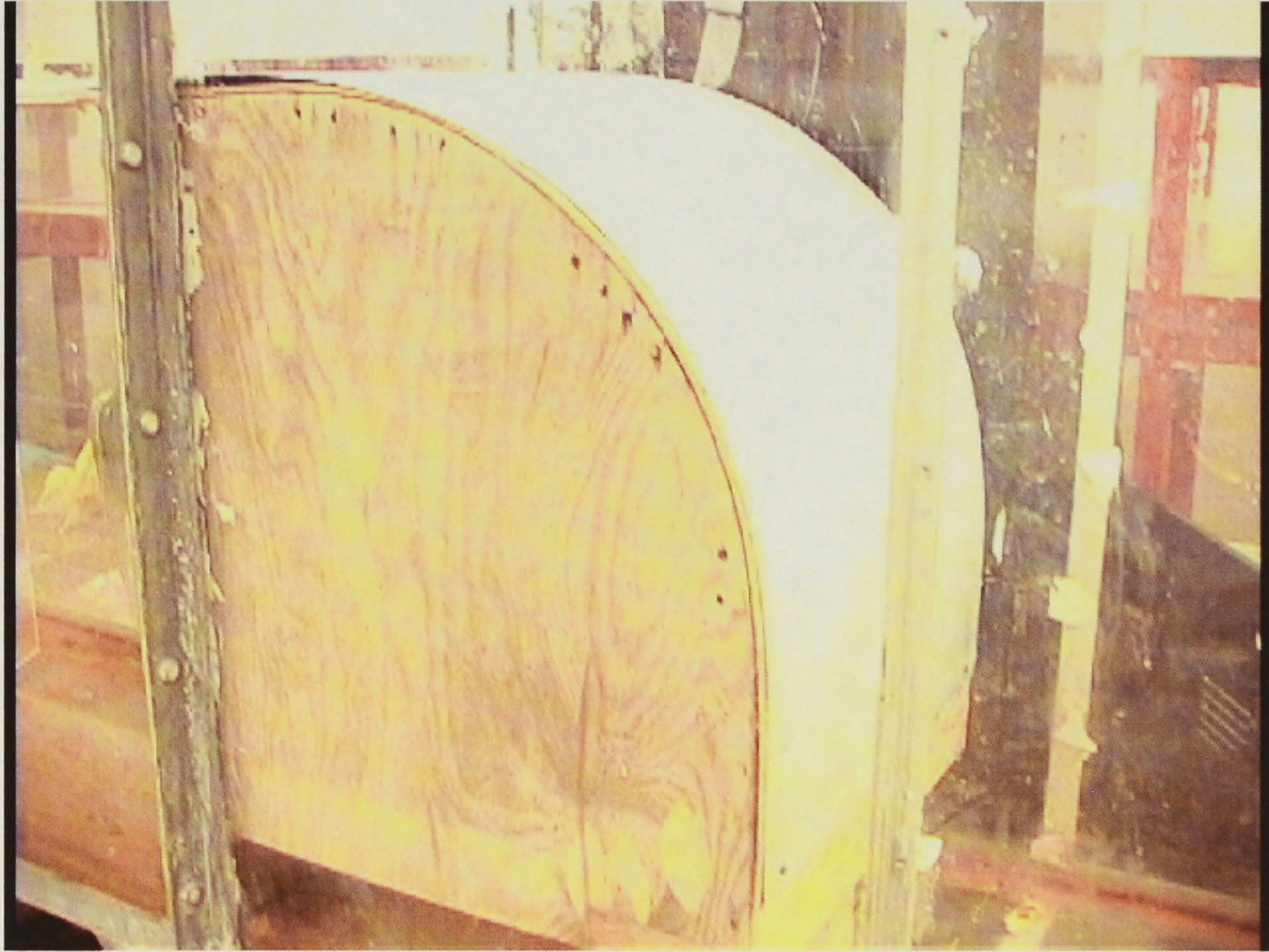
Figure 8: Two-Dimensional Flume Model to Study Overfall Condition.
