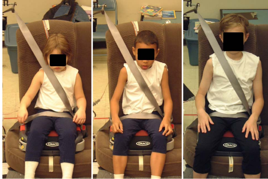
Figure 32. Children with a range of stature in trials with shoulder belt score within one mm of the ideal SBS calculated from equation 5.
