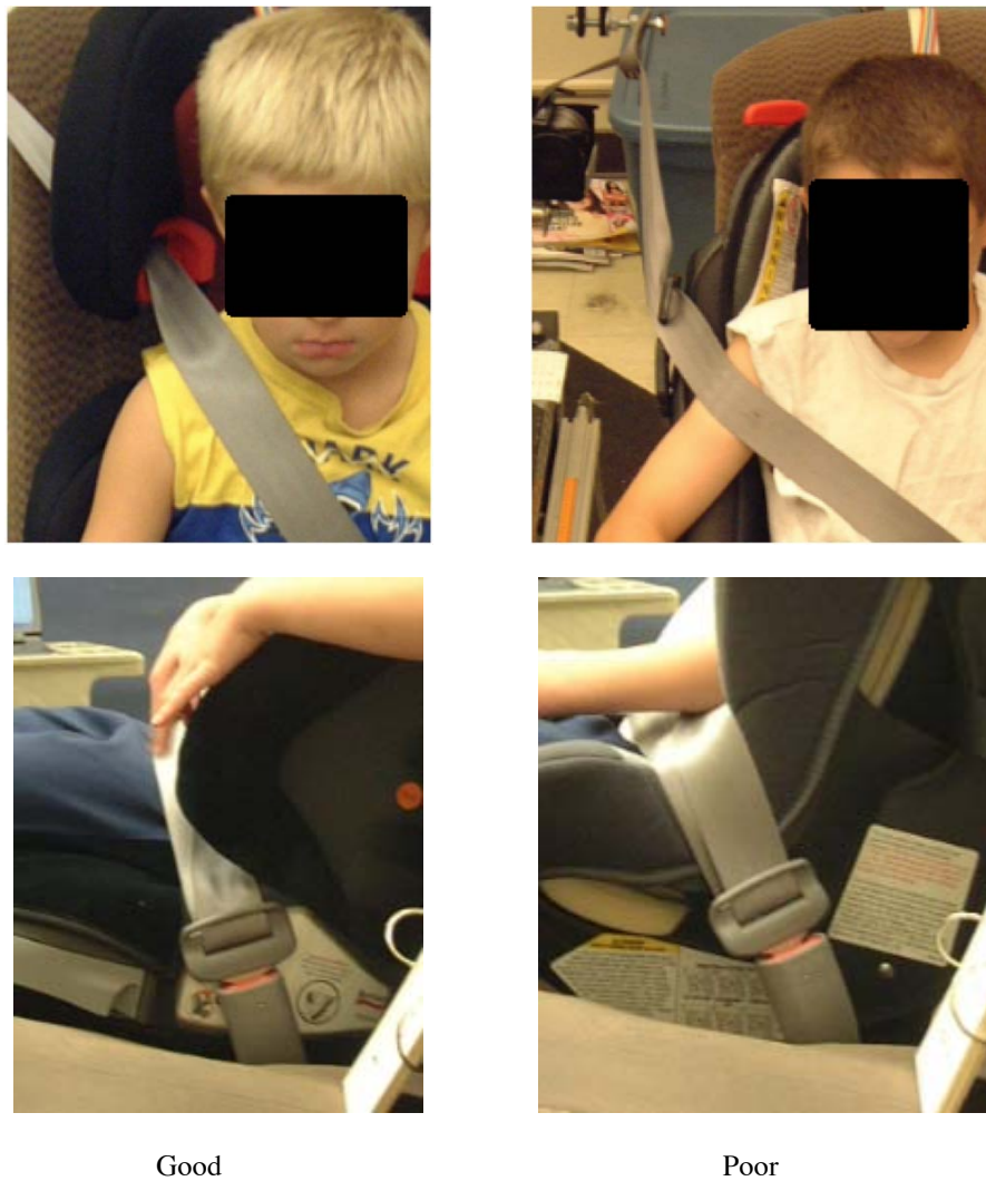
Figure 34. Illustration of good (left) and poor (right) belt routing guide designs for the shoulder portion of the belt (top) and lap portion (bottom).
