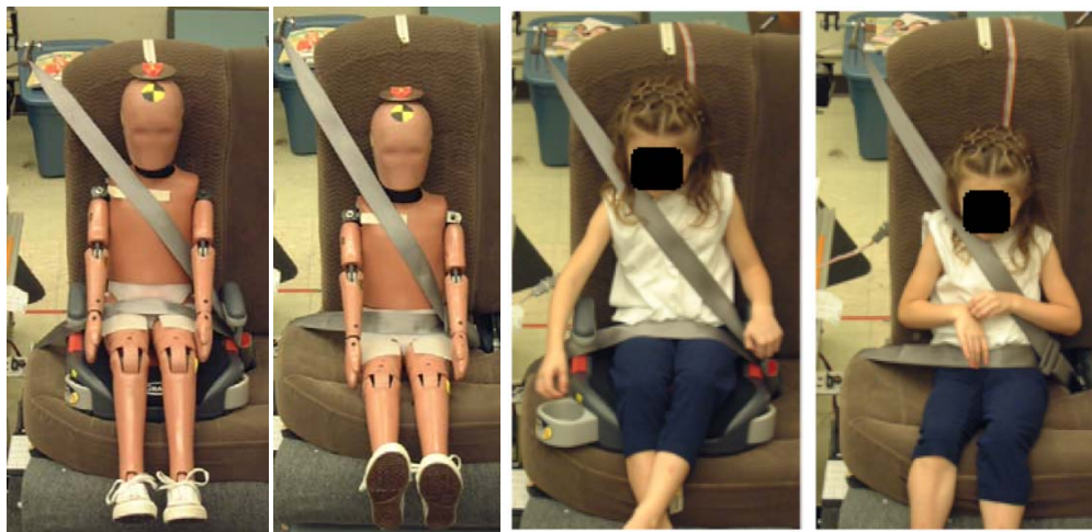
Figure 30. Comparison of shoulder belt fit for the 6YO ATD and one child in the backless TurboBooster and no-booster conditions, showing the effect of slumping on sitting height for the child.
