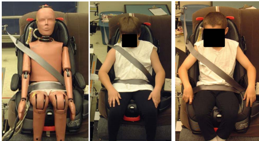
Figure 31. Comparing shoulder belt routing for the 10YO ATD and two large children in the Alpha Omega.
