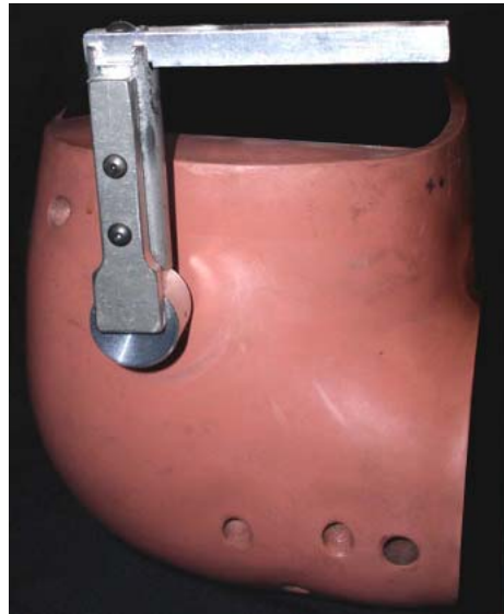
Figure B3. Removable pelvis measurement fixture.
