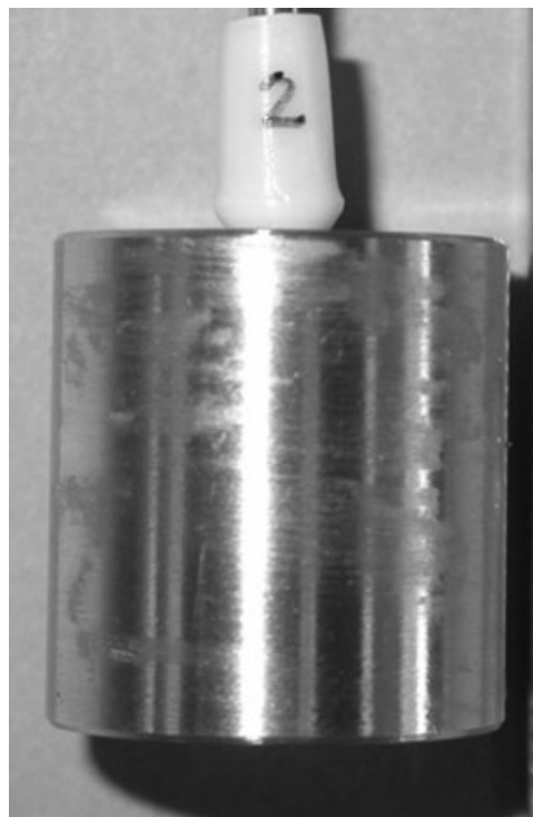
Figure 1 Abutment assembly fixed within implant analog with Field's metal. The analog was fixed flush with the top of the stainless steel cylinder and held in place with Field's metal. The prepared abutments were then screwed in place with the screw provided and torqued to 25 Ncm. This is now considered the "assembly."
