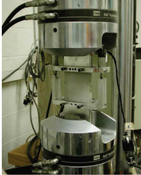
Fig. 3 Setup of the uniaxial tensile test
