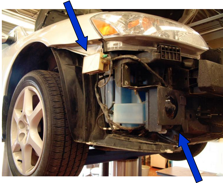
Figure A.3 Physical installation of the forward and side radars. (Reproduced from [53])
