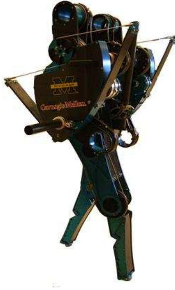
Figure 1.1: MABEL, an experimental testbed for bipedal locomotion. The robot is planar, with a boom providing stabilization in the sagittal plane. The robot’s drivetrain contains springs for enhanced power efficiency.
