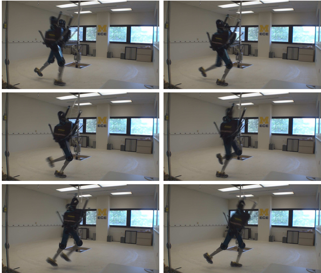
Figure 7.2: Typical running step for MABEL with feet. Snapshots are at an interval of 100 ms.
