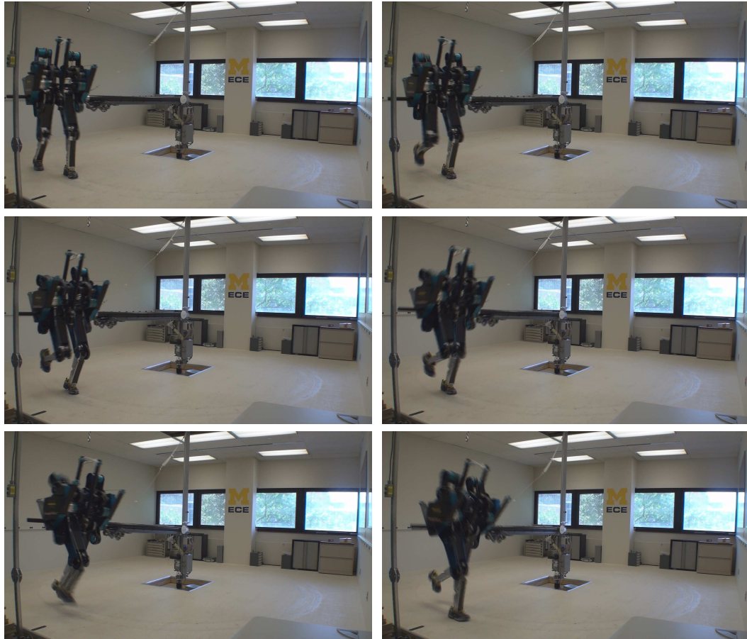
Figure 7.1: Transitioning from walking to running for MABEL with feet. The first step of the transition and the transition from the transition-walk-step to a transition-run-step is shown. Snapshots are at an interval of 100 ms.
