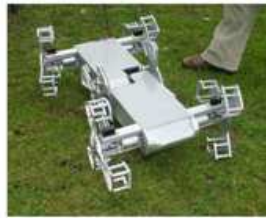
Figure 2.19 Whegs: Production-ready Robot from Roger Quinn's Group
