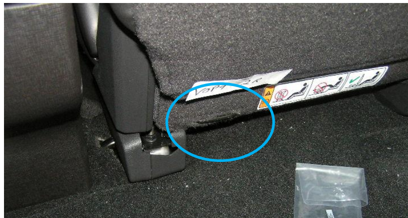
Figure 47. Representative unmarked tether anchorage often found in minivans/crossover vehicles.
