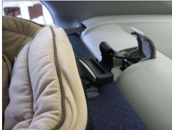
Figure 48. Tether anchorage located too close to allow space to tighten tether.
