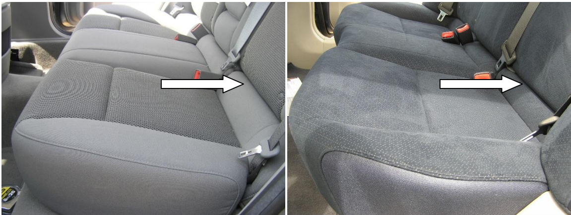
Figure 9. Illustration of vehicle seats with a bightline waterfall with vertical lower anchorage locations indicated.
