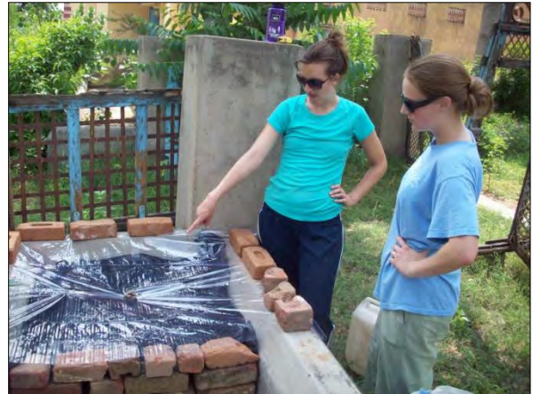
COCO (Bagar): Lined evaporation basin and catchment hood for evaporation tests (07/19/11)
