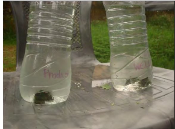
Algae Bench Test: Algae in product (right) and source water (left) bottles (08/05/11)
