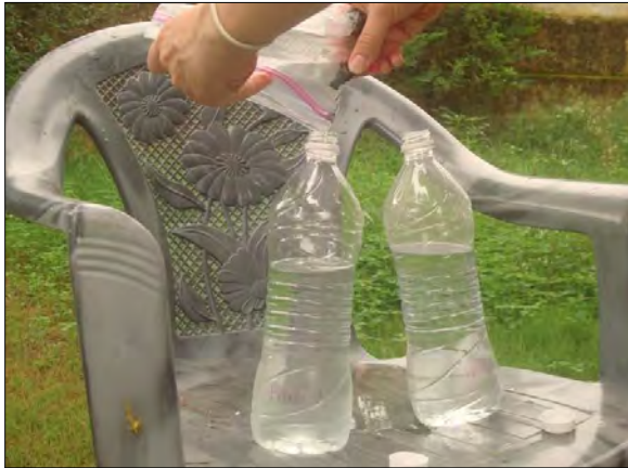
Algae Bench Test: Placing algae in RO brine and source water bottles (08/05/11)
