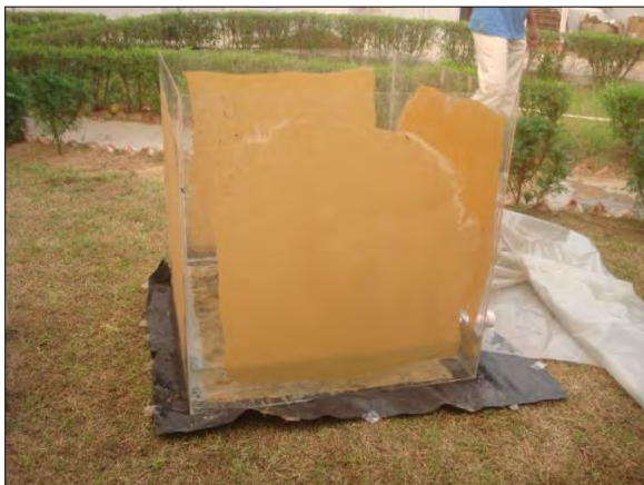
Evaporation Bench Test: Acrylic basin filled with RO brine (08/05/11)
