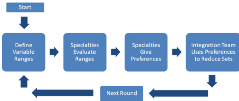
Figure 3: Overview of the Design Process
