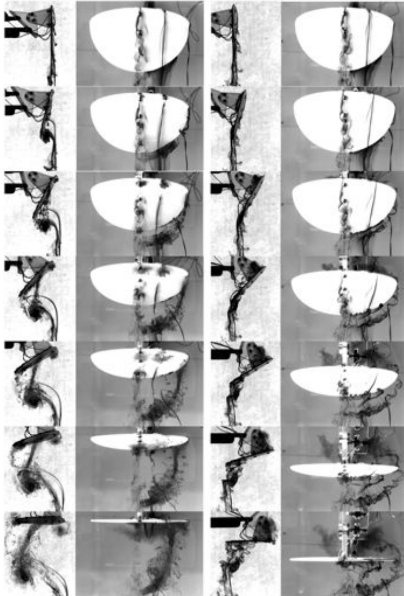
Figure 7. Side- and planform view of Zimmerman AR=2 plate pitching at K = 1.0 , with pivot at leading edge (left) and trailing edge (right). Snapshots at incidence angles of 0^\circ , 15^\circ , 30^\circ , 45^\circ , 60^\circ , 75^\circ and 90^\circ .
