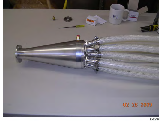
Figure 27. Optical cable assembly designed and utilized by Physical Sciences Inc.
