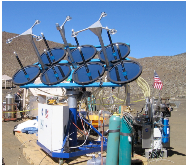
Figure 18. Photograph of the Solar Concentrator Array (left) with the Carbothermal Regolith Reduction Module hardware (right).
