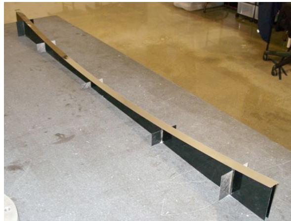
Figure 12. Implementation of Fresnel mirror on composite rib, and assembled on a positioning tool using a frame that fixed the mirror strip position.
