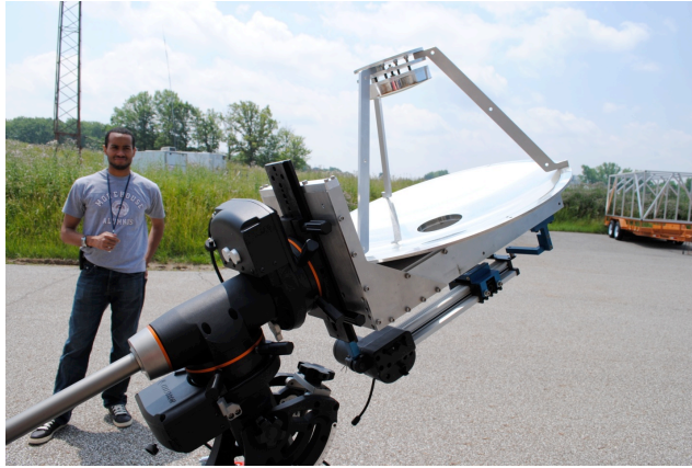
Figure 2. Pierce Gordon standing next to a Cassegrain concentrator manufactured for NASA GRC.
