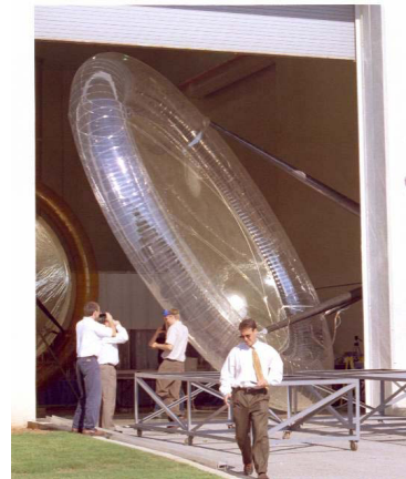
Figure 23. Flexible 4 m by 6 m offset parabolic concentrator.
