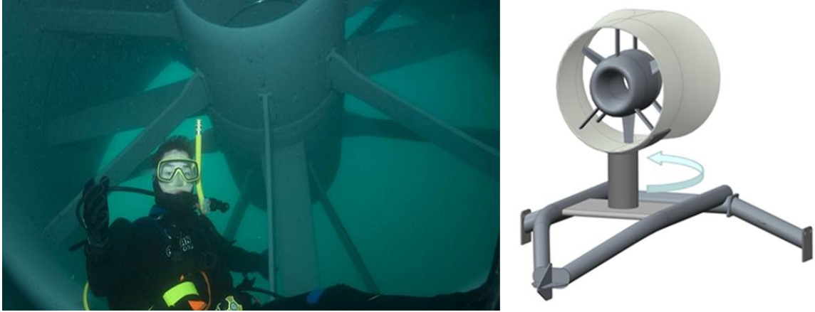
Figure 1.9: Demonstration Prototype installed in 2006 and schematic of Tidal Turbine [Reproduced from www.cleancurrent.com ]
