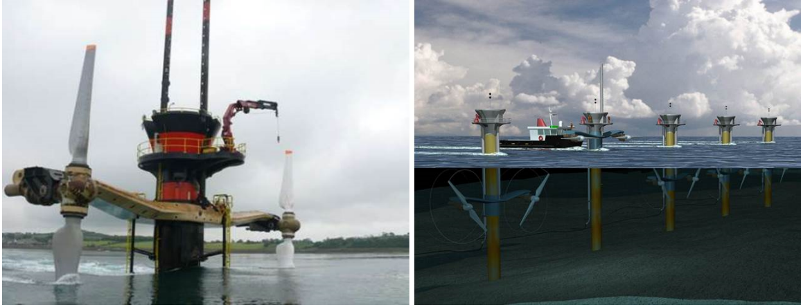
Figure 1.8: 1.2M Test prototype installed in 2008 (left) and schematic of the SeaGen [Reproduced from www.seageneration.co.uk ]
