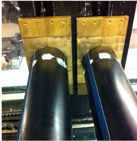
Figure 7.27: Additional mass attached at the end of the two cylinders
