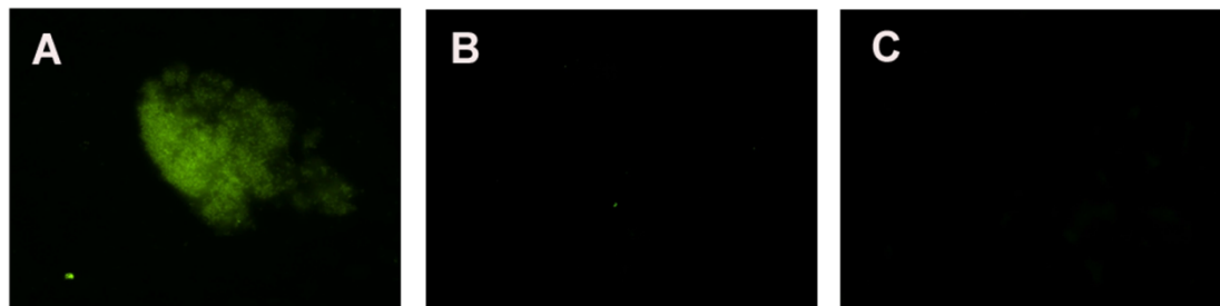
Figure 3.20. Fluorescent micrographs of E. Coli biofilm on the surface of A) glass slide; B) (PEI/Alg) 50 ; C) (e-PEI/Alg) 50 after 7 d antibiofilm test in a CDC biofilm reactor, E. Coli was labeled by green fluorescence protein (GFP).
