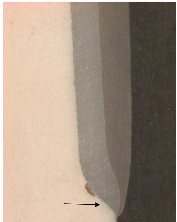
Figure 26. Sectioned crown (Design 3 - lingual surface) at 20X magnification
