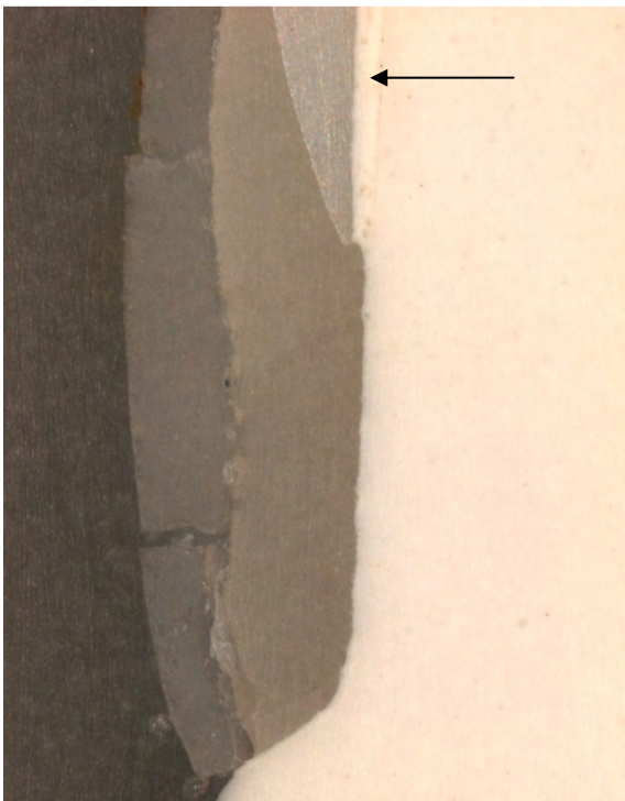
Figure 25. Sectioned crown (Design 3 - facial surface) at 20X magnification
