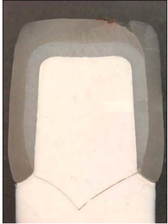
Figure 21. Sectioned crown (Design 2) at 10X magnification
