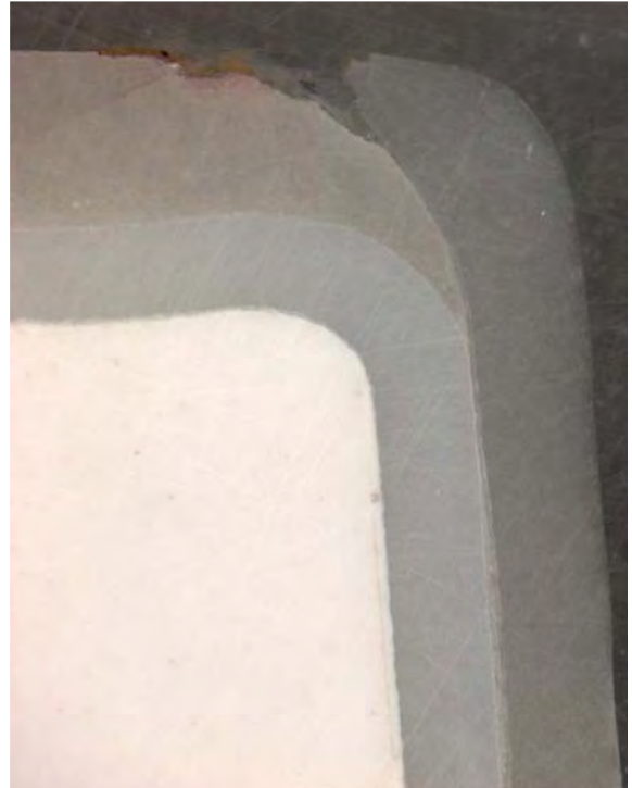
Figure 28. Sectioned crown (Design 2 - axio-occlusal surface) at 20X magnification
