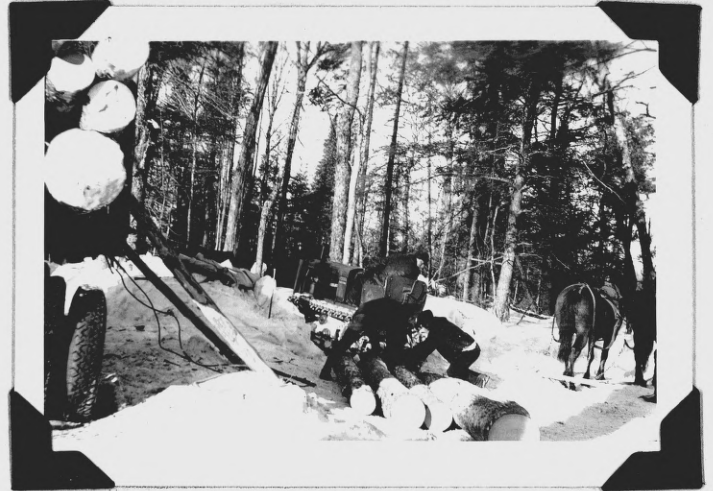
Unhooking logs from tractor at skidway
