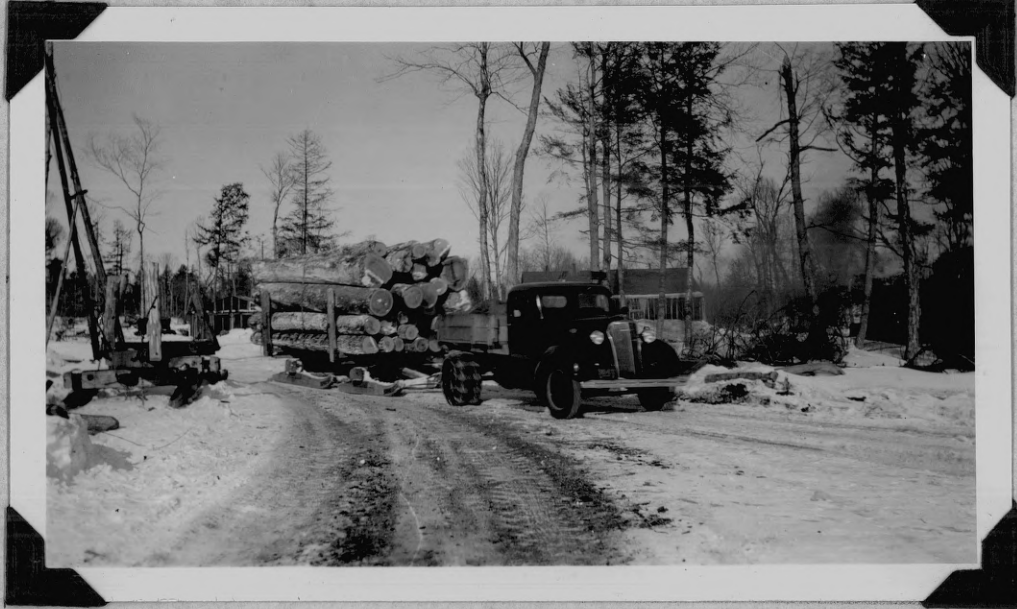
Chevrolet 1 \frac{1}{2} Ton Truck Drawing Sleigh Carrying 2,000 M Note that back of truck is filled with sand bags.
