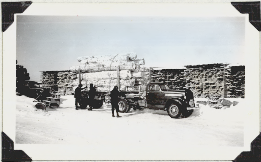
Trucks with rated capacity of 2-3 tons carry loads of 2,000 Mbm of hardwoods and 3,000 Mbm of pine.
