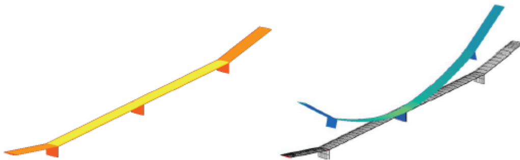
Figure 3.2: Comparison of trimmed shape for 0-kg (left) and 227-kg (right) center payloads to undeformed shape (black mesh) [1]
